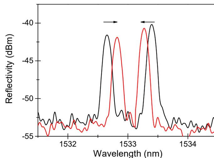
**Figure 17.** Reflection spectra of an FBG written in a highly birefringent PCF, unstressed (black curve), and when a transverse load is applied (red curve). The arrows highlight the direction of the shift in the peaks.
