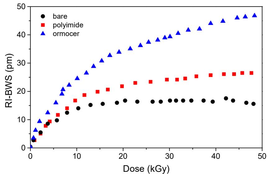
**Figure 15.**  $\gamma$ -rays induced BWS as a function of the dose, for identical type I FBGs written with a UV laser (at 248 nm, a pulse width of 15 ns, and power energy of 400 mJ/cm<sup>2</sup>) in a highly Ge-doped fiber and recoated after inscription with polyimide (which was thermally cured) or ormocer, with a dose rate of  $\sim 0.11$  Gy/s, at 35 °C. A bare grating was also reported for the sake of comparison. Data extracted from [108].
