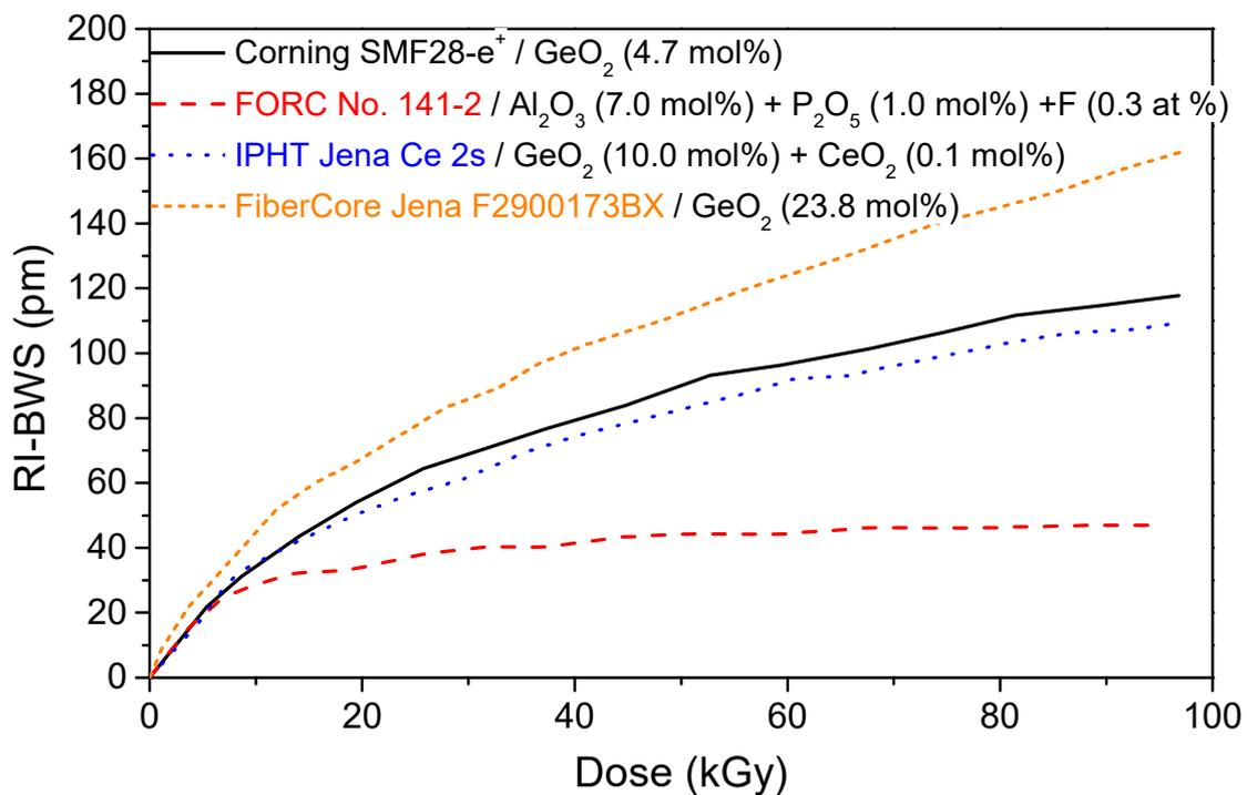
**Figure 4.** BWS induced by  $\gamma$ -rays on type I-UV gratings, written by different manufacturers on uncoated fibers with different core compositions that were recoated after inscription, the dose rate being 0.9 Gy/s up to 100 kGy at RT. Data extracted from [76].
