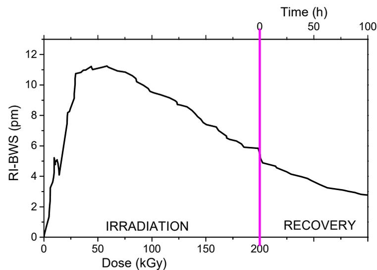
**Figure 11.**  $\gamma$ -rays-induced Bragg wavelength shift on type I FBGs, inscribed with an ns-pulsed UV laser (at 248 nm, a pulse width of 15 ns, and pulse energy of 8 mJ) in an unloaded highly Ge-doped core (~8 mol% of GeO<sub>2</sub>). The vertical pink line indicates the irradiation end. The accumulated dose reached in the only first irradiation run, here reported, was around 200 kGy, the dose rate being of about 0.28 Gy/s and a temperature of about 34 °C. Data extracted from [92].
