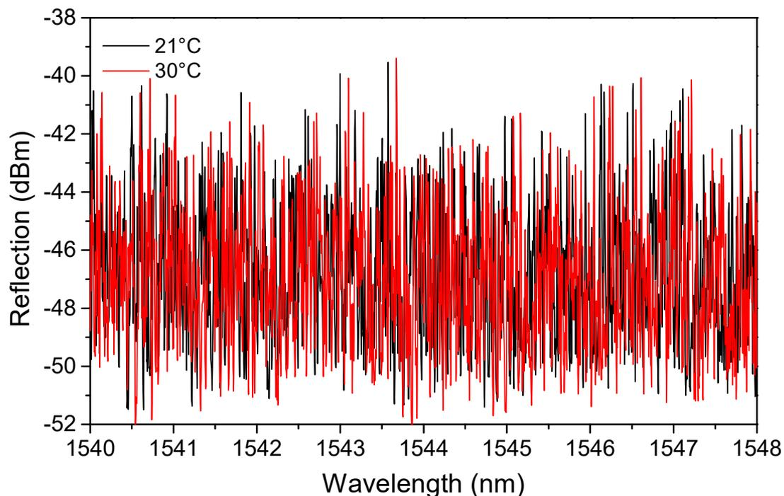
**Figure 16.** A part of reflection spectra of a type II 10 cm long FRG, inscribed in a Ge-doped fiber (the Corning SMF28e) with an fs-laser (at 800 nm), acquired at two temperatures, in order to highlight the changes induced by a temperature variation of about 10 °C. Data extracted from [114].
