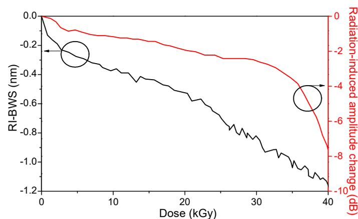
**Figure 19.** RI-BWS on the left (black curve) and peak amplitude reduction on the right (red curve) as a function of the dose, for an FBG written with an fs-laser in a CYTOP, under  $\gamma$ -rays. Data extracted from [38].
