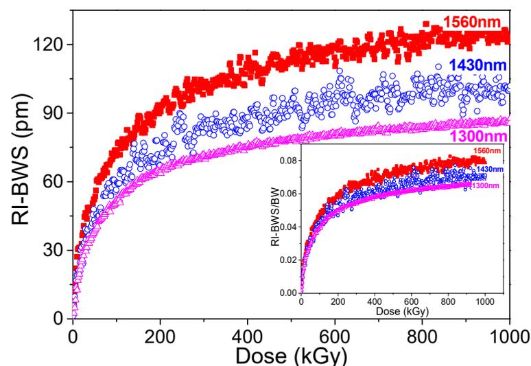
**Figure 8.** BWS induced by X-rays at RT up to 1 MGy (dose rate of 50 Gy/s) on three similar gratings (having the same  $\Delta n^{\text{mod}}$  of about  $2 \times 10^{-4}$ ) written with a CW UV laser (at 244 nm) in  $\text{H}_2$ -loaded Corning SMF28 at different Bragg wavelengths. In the inset, RI-BWS normalized with respect to the initial Bragg wavelength. Data extracted from [49].
