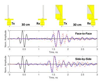
FIGURE 12. Measured and simulated Tx and Rx signals of the proposed antenna: input (solid-black), simulated (solid-blue), measured (dash-red).
