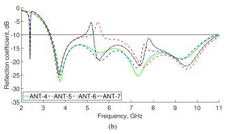
FIGURE 3. Effect of structural modifications shown in Fig. 2 on the antenna input reflection coefficient: (a) ANT-1 to 4, (b) ANT-4 to 7.
