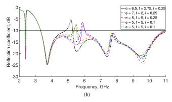
**FIGURE 8.** Simulated antenna input reflection coefficients as a function of the slits parameters: (a)  $S_1$ , (b)  $S_2$ .
