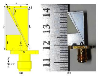
**FIGURE 1.** Proposed antenna: (a) schematic geometry used in the simulation, (b) prototype photograph; a=10 mm, b=20 mm, c=1.4 mm, d=18.8 mm, e=6.5 mm, f=2.75 mm, g=0.2 mm, i=0.25 mm, j=0.2 mm, k=16.5 mm, k=3 mm, k=16.5 mm, k=
