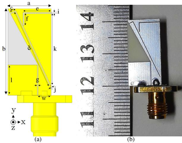
**FIGURE 1.** Proposed antenna: (a) schematic geometry used in the simulation, (b) prototype photograph;  $a = 10$  mm,  $b = 20$  mm,  $c = 1.4$  mm,  $d = 18.8$  mm,  $e = 6.5$  mm,  $f = 2.75$  mm,  $g = 0.2$  mm,  $i = 0.25$  mm,  $j = 0.2$  mm,  $k = 16.5$  mm,  $w = 3$  mm,  $l = 7$  mm.
