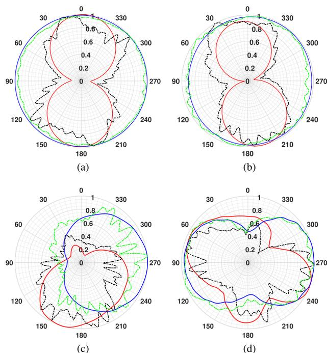
**FIGURE 10.** Measured and simulated normalized radiation patterns of the proposed antenna at: (a) 2.4 GHz (lower passband frequency), (b) 3.7 GHz (middle passband frequency), (c) 4.9/5.2 GHz (stopband frequency), and (d) 9.5 GHz (higher passband frequency). Dashed-black (solid-red) and dashed-green (solid-blue) are the measured (simulated) *E*- and *H*-plane, respectively.
