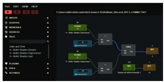
Fig. 3. CONNECT I/O: soft PLC for HOME I/O
