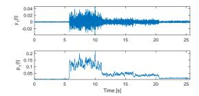
Fig. 6. Illustration of estimated index activity from actual sEMG signal. On top: best estimated component. On bottom: its related instantaneous power.
