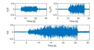
Fig. 2. Artificial mixture of one electrode on the 64. Top left (res. right): signal  $s_I(t)$  (resp.  $s_{LF}(t)$ ) corresponds to the extension of the index (resp. little finger) alone. Bottom: artificial mixture  $x(t=s_I(t)+s_{LF}(t))$ .
