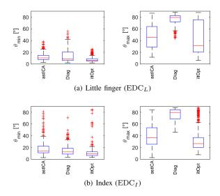
Fig. 4. Performance of separation to extract the little finger (Fig. 4(a)) and index (Fig. 4(b)). In each figure, the minimum (left) and maximum (right) angles are presented for each method. Each box plot shows the median as central red line, the bottom and top edges are the 25th and 75th percentiles, respectively. The whiskers extend to extreme values and the outliers are plotted as red crosses.
