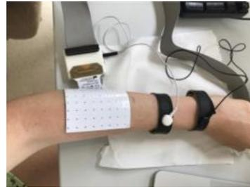
Fig. 1. The 64-channel electrode grid (8x8 channels, 10 mm inter-electrode-distance) used to record the sEMG activity from extensors of index and little finger
