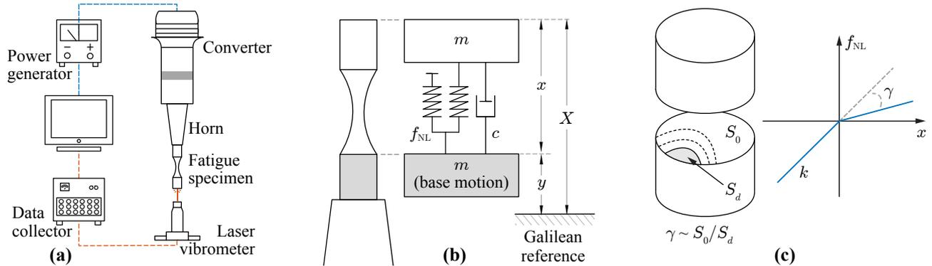
Figure 1: (a) Schematic of ultrasonic fatigue test experimental setup, (b) fatigue specimen model with absolute displacement of mass  $X$  and Galilean reference displacement for mass  $x$  and base  $y$ , and (c) concept of crack nonlinearity parameter  $\gamma \sim S_d/S_0$  with plot of the bilinear stiffness restoration force  $f_{NL}$ .
