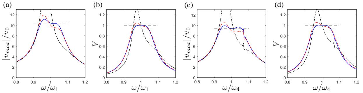
**Figure 6:** FRP for displacement and voltage around the (a)+(b) first and (c)+(d) fourth resonant frequency for parallel shunt tuning based on the effective Eq. (13) (solid line), quasi-static Eq. (19) (dashed line) and modal Eq. (15) (dashed-dotted line) EMCC in respect to mode  $r$ .
