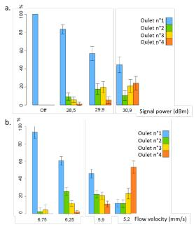
Fig. 6. Collected cells distribution at each sorting system outlets as function of (a) the signal power at constant speed flow of  $4.7 \text{ mm.s}^{-1}$ ; (b) the flow velocity at constant signal power of 29.9 dBm. The signal frequency was 500 MHz. The bars represent the standard error of mean.
