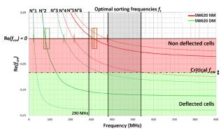
Fig. 4. Theoretical plot of the real part of the CM factor as a function of the frequency and according to the measured dielectrophoretic signatures for the SW620 NM (red curves) and SW620 DM (green curves) from Fig.1. The critical  $f_{cm}$  is determined over a range of possible values for an angle  $\theta$  of 10°, considering the electrodes are biased with a signal magnitude of 37.7 dBm and a fluid flow velocity in the microchannel 7 mm.s<sup>-1</sup>.
