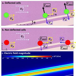
Fig. 3. (a) and (b) Working principle of selective cell trajectory deviation related to intrinsic cell dielectric intracellular properties. With  $F_{DEP}$  is the DEP force,  $F_D$  the Drag force,  $\alpha$  the deflection angle of the cell trajectory and  $\theta$  the electrodes slope. (c) COMSOL Multiphysics numerical simulation of the electric field b considering a applied voltage of 5Vpp between electrodes.
