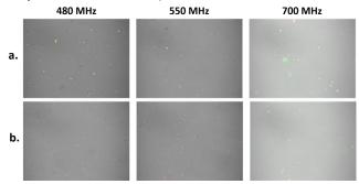
Fig. 8. Optical photographs of collected cells at outlet n°1 (b) and outlet n°2 (a) of the dielectrophoretic cytometer biased at different signal frequencies. Green cells are SW620 DM and red cells are SW620 NM.
