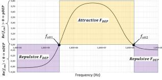
Fig. 2. Plot of the real part of the CM factor of a biological cell with its two dielectrophoretic signatures  $f_{x01}$  and  $f_{x02}$ .
