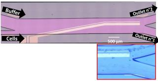
Fig. 7. Second dielectrophoretic cytometer prototype design: focus on the sorting area. The red frame represents the cytometer during a sorting experiment.
