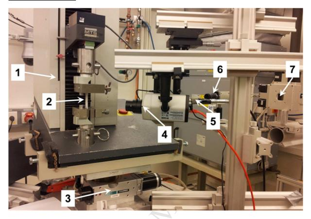
Special experimental set up developed to perform simultaneous high energy wide angle X-rays scattering (P07 beamline, PETRA III, DESY synchrotron, Hamburg, Deutschland) and Raman spectroscopy analysis during a mechanical tensile test: 1) Tensile test machine, 2) Dumbbell-shape specimen, 3) Z-motorized stage, 4) Video camera, 5) Raman head of probe, 6) VidéoTraction<sup>TM</sup> camera, 7) X-rays monochromator.
