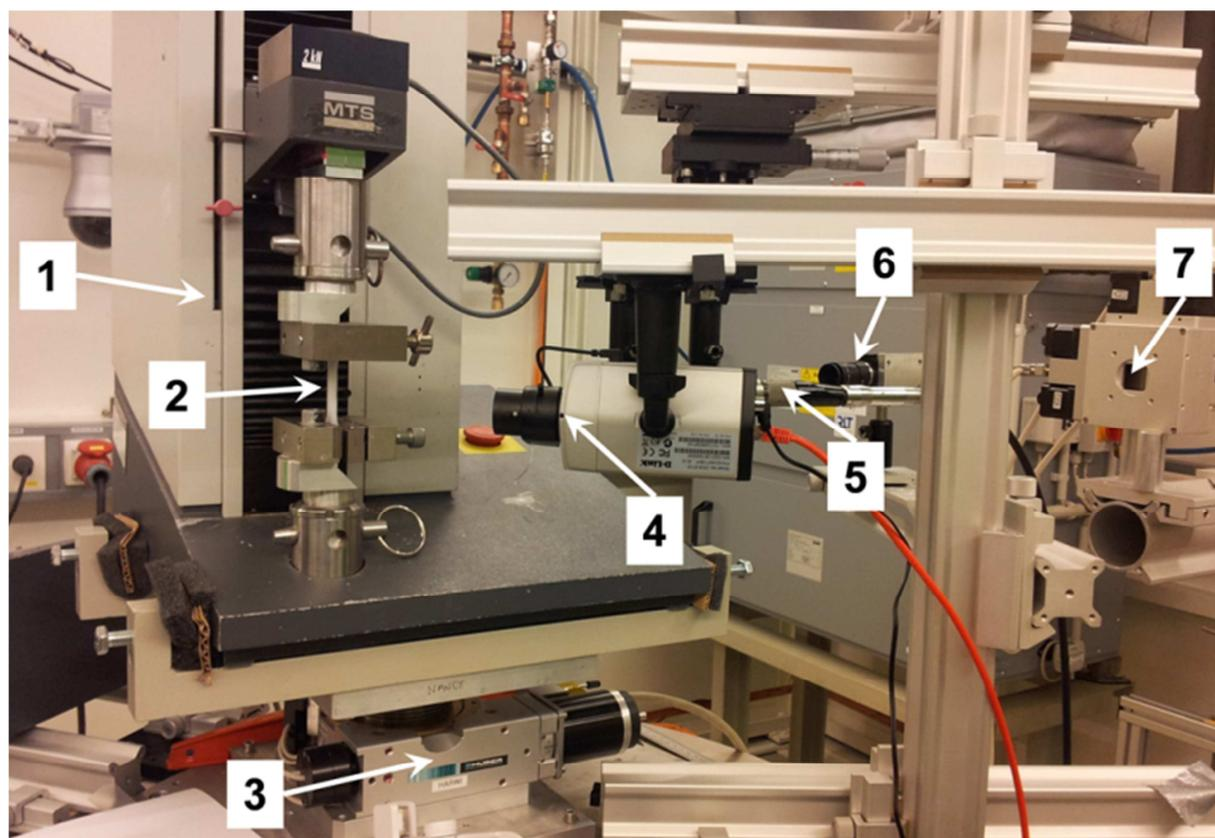
Special experimental set up developed to perform simultaneous high energy wide angle X-rays scattering (P07 beamline, PETRA III, DESY synchrotron, Hamburg, Deutschland) and Raman spectroscopy analysis during a mechanical tensile test: 1) Tensile test machine, 2) Dumbbell-shape specimen, 3) Z-motorized stage, 4) Video camera, 5) Raman head of probe, 6) VidéoTraction™ camera, 7) X-rays monochromator.
