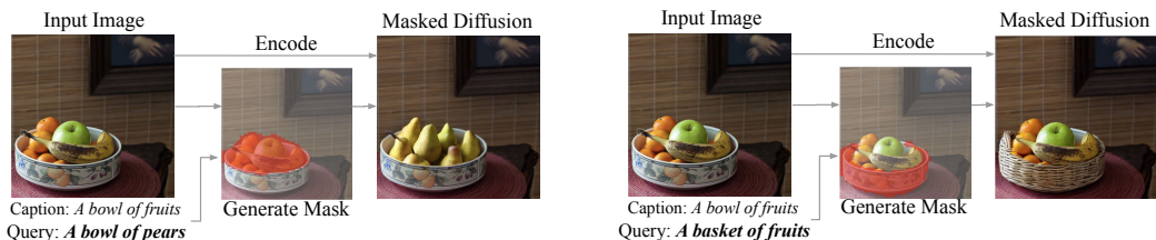
Figure 1: In semantic image editing the goal is to modify an input image based on a textual query, while otherwise leaving the image as close as possible to the original. In our DIFFEDIT approach, a mask generation module determines which part of the image should be edited, and an encoder infers the latents, to provide inputs to a text-conditional diffusion model which produces the image edit.
