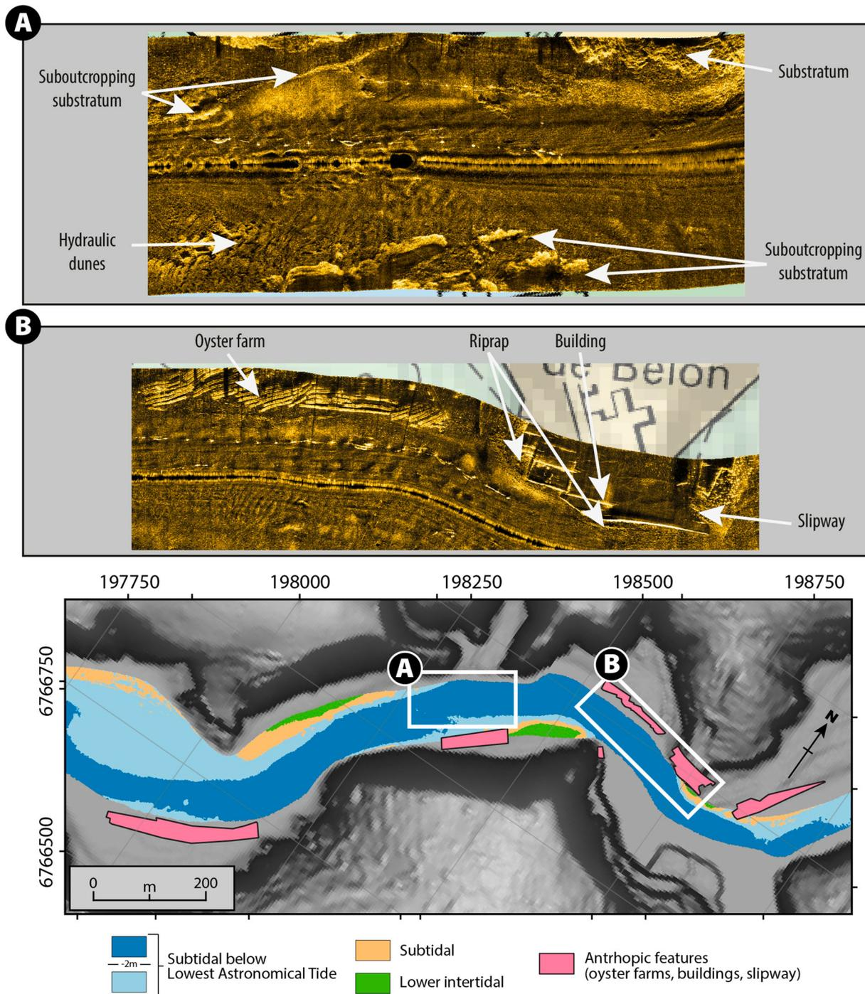
**Figure 3.** Sampled side-scan sonar mosaic exhibiting: (A) natural features, such as outcropping and sub-outcropping substratum, hydraulic dunes, and (B) anthropic features such as mooring lines, slipways, buildings and oyster farms. Both sampled mosaics are located on the classified bathymetric map based on the French hydrographic datum with the location of the interpreted substratum (in red) and location of the main anthropic features (in pink).
