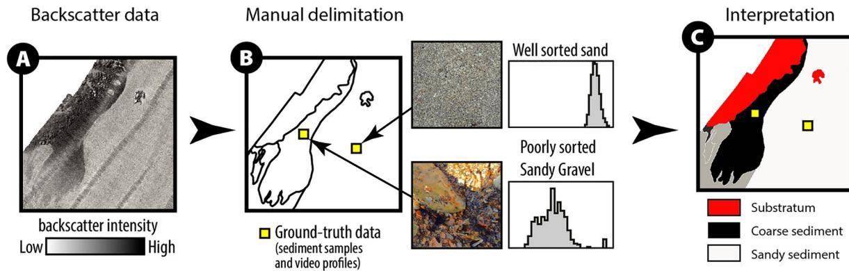
**Figure 1.** Production process of the sediment map based on: (A) the backscatter data, and (B) the manual delimitation of the acoustic facies and their characterisation using sediment samples and videos, to (C) interpret the sediment classes.
