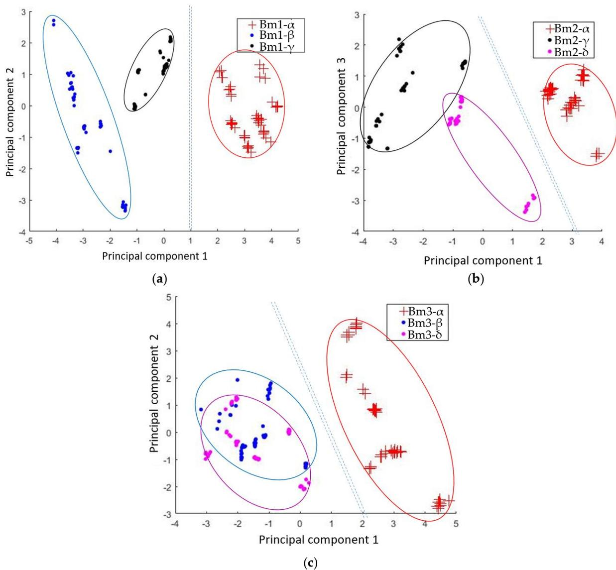
**Figure 7.** First principal component as a function of second principal component for signals received in sensor #2 (a) beam #1 (b) beam #2 (c) beam #3.
