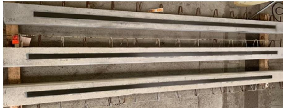
Figure 1. Samples of composite/RC-beam adhesively bonded assemblies.
