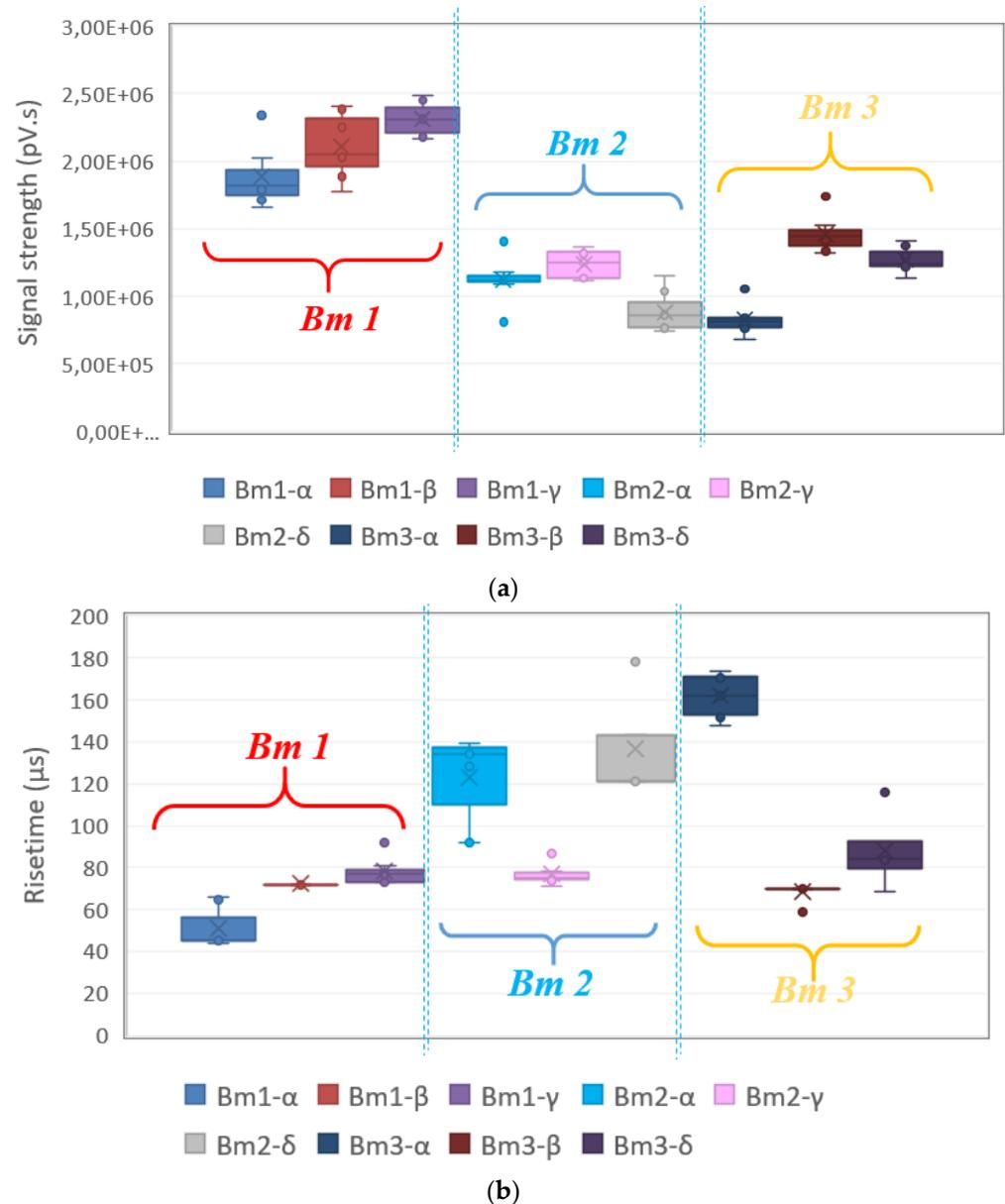
**Figure 4.** Parametric analysis of the signals recorded by sensor #1. (a) Signal strength (pV.s): Integral of the rectified voltage signal over the duration of the AE waveform and (b) risetime (µs): time between the first threshold crossing and the peak amplitude of the signal.
