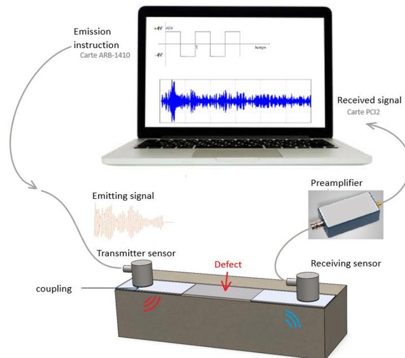
**Figure 3.** Experimental setup for acousto-ultrasonic measurements.
