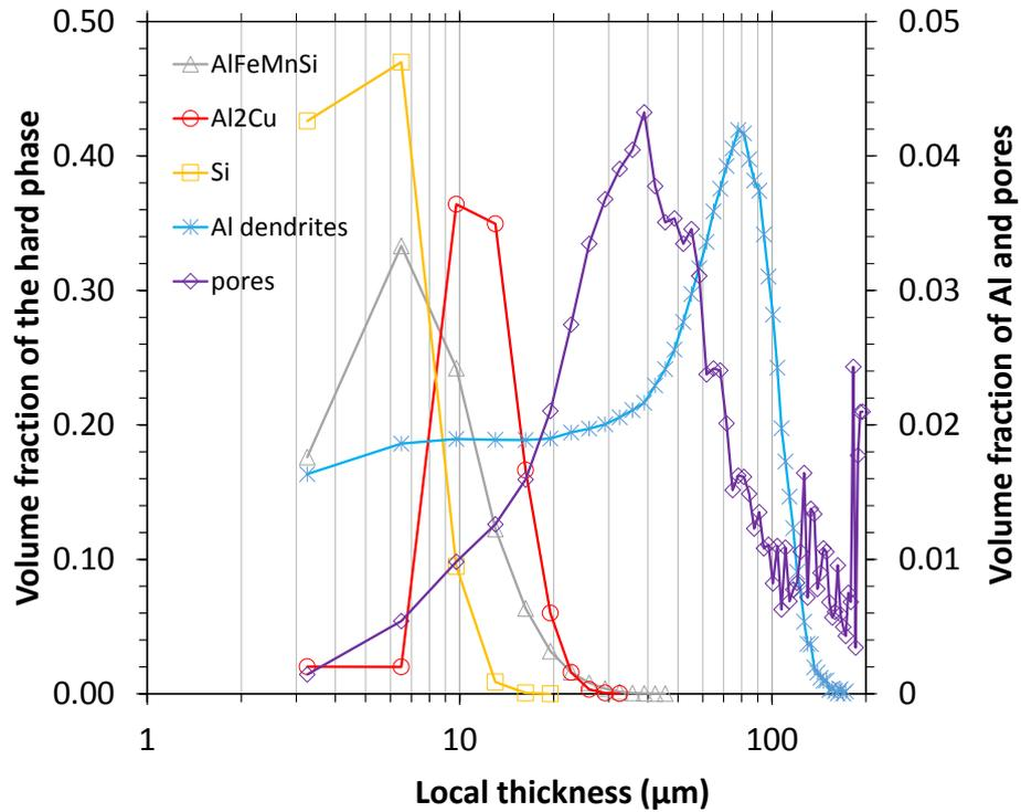
**Figure 4 :** Thickness distribution in volume fraction of the considered phase; Analysis is based on tomography images with a 1.6 μm voxel size hence objects thinner than 3.2 μm are not included.
