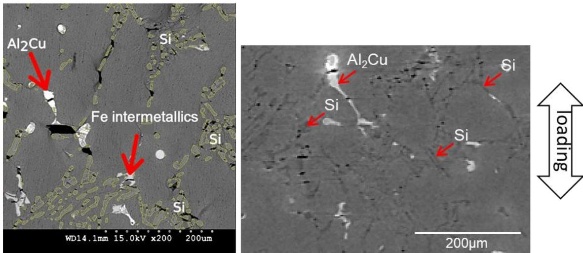
**Figure 6: Comparison of broken hard particles observed post-mortem at the surface with SEM where the Si phase contour is underlined in yellow (on the left) and in the bulk with X-ray tomography at the last scan before failure (on the right). The two images are shown at comparable magnification.**
