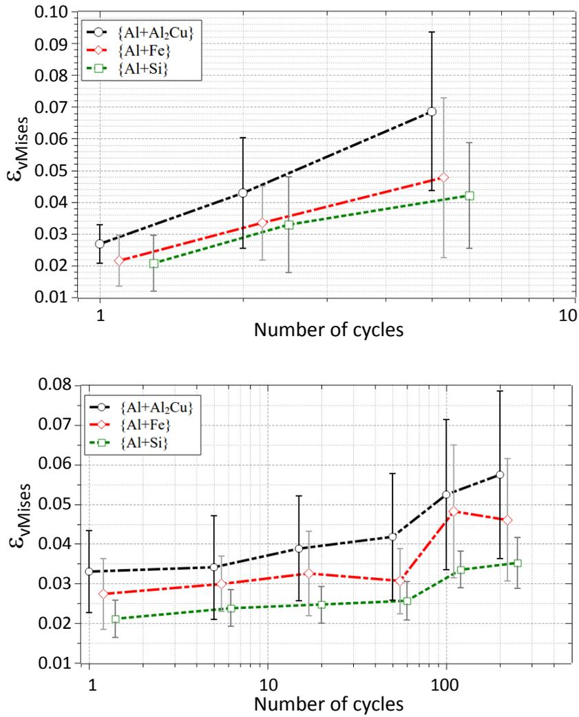
**Figure 10: Mean evolution of the  $\epsilon_{vMises}$  strain before failure for the three types of hard particles in specimen A4 (top) and LE7 (bottom) that failed after 50 and 1,800 cycles, respectively; the three series are shifted on the abscissa to improve readability of the figure.**
