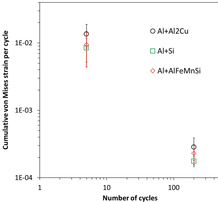
**Figure 11 : Manson-Coffin curves of the different hard phases at 250°C.**
