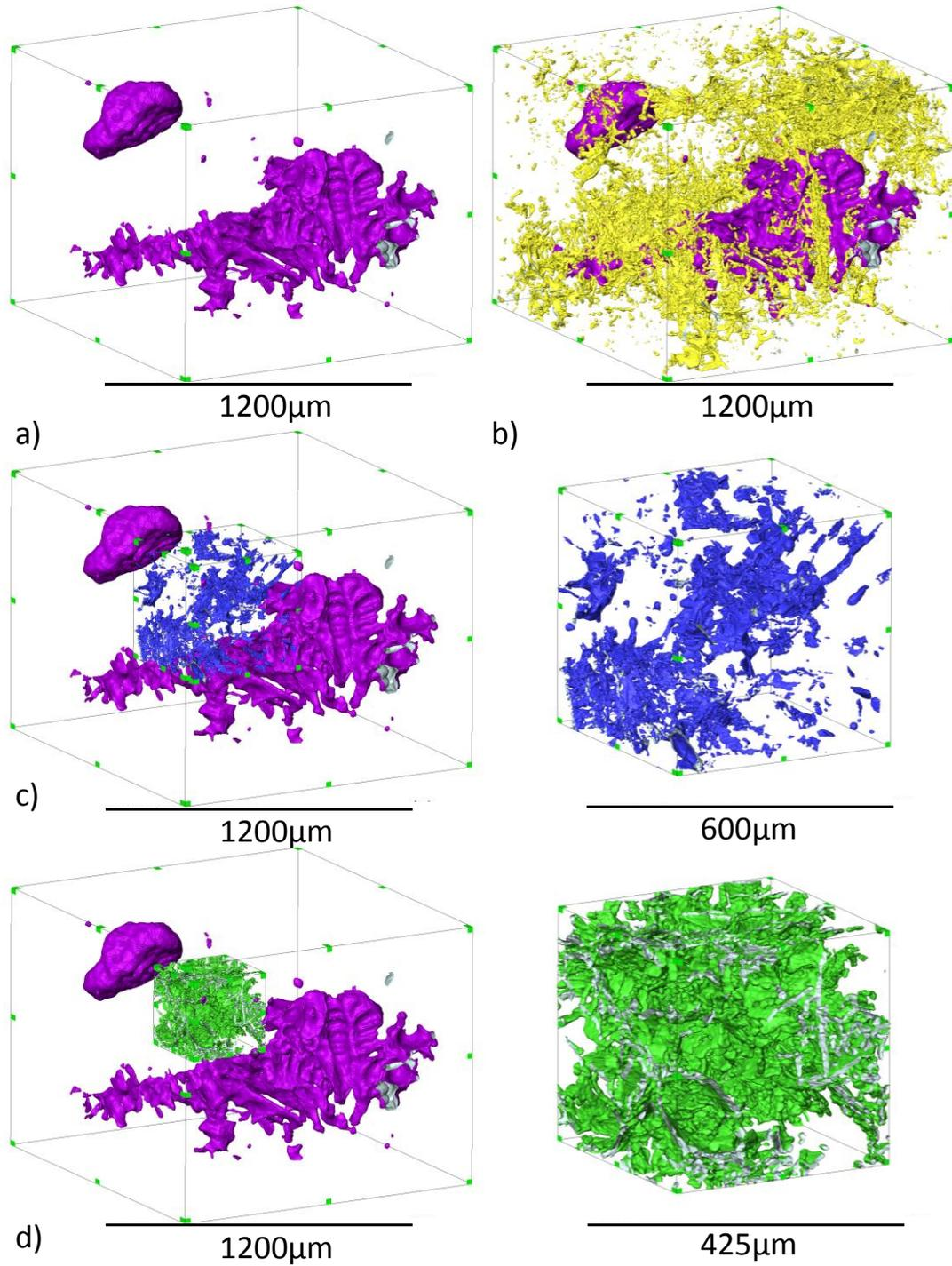
**Figure 3: 3D microstructure of AlSi7Cu3Mg using high resolution tomography (voxel=1.6µm) showing (a) pores and hard phases: (b) Al<sub>2</sub>Cu, (c) Al(Fe,Mn)Si and (d) Si; For the thin Al(Fe,Mn)Si**
