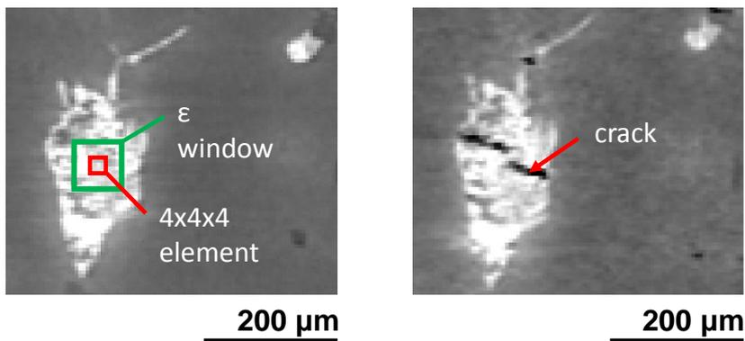
**Figure 5:** Illustration of the spatial resolution of local measurement (on the left, in red for displacement and in green for strain) in an Al-Al<sub>2</sub>Cu particle that eventually breaks (on the right)
