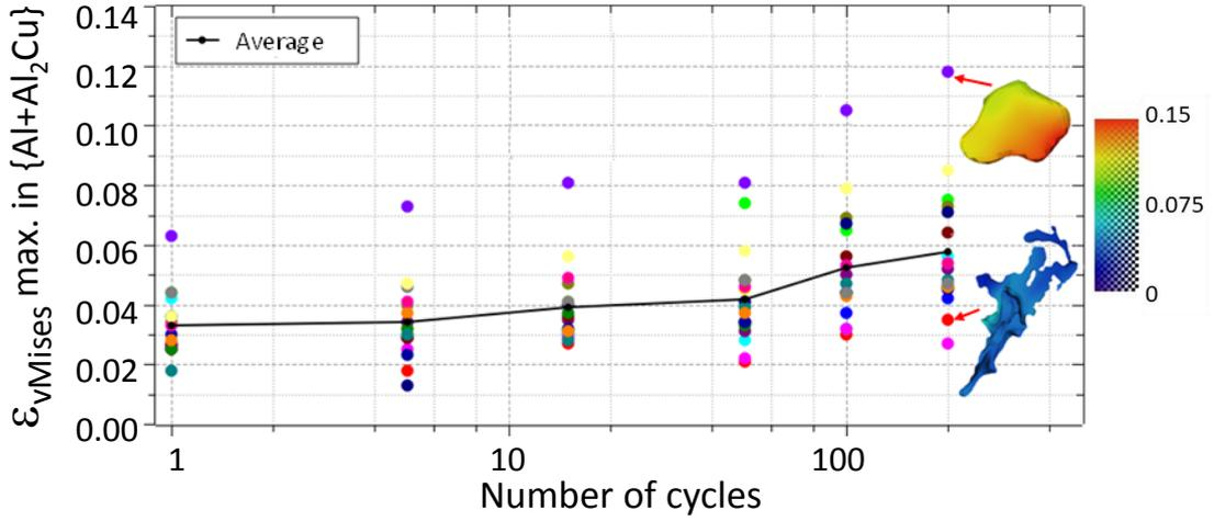
**Figure 9: Evolution of the  $\epsilon_{vMises}$  strain within several  $\{Al+Al_2Cu\}$  particles with the number of cycles up to failure (sample LE7). A 3D rendering shows the strain localization at 200 cycles for two particles.**
