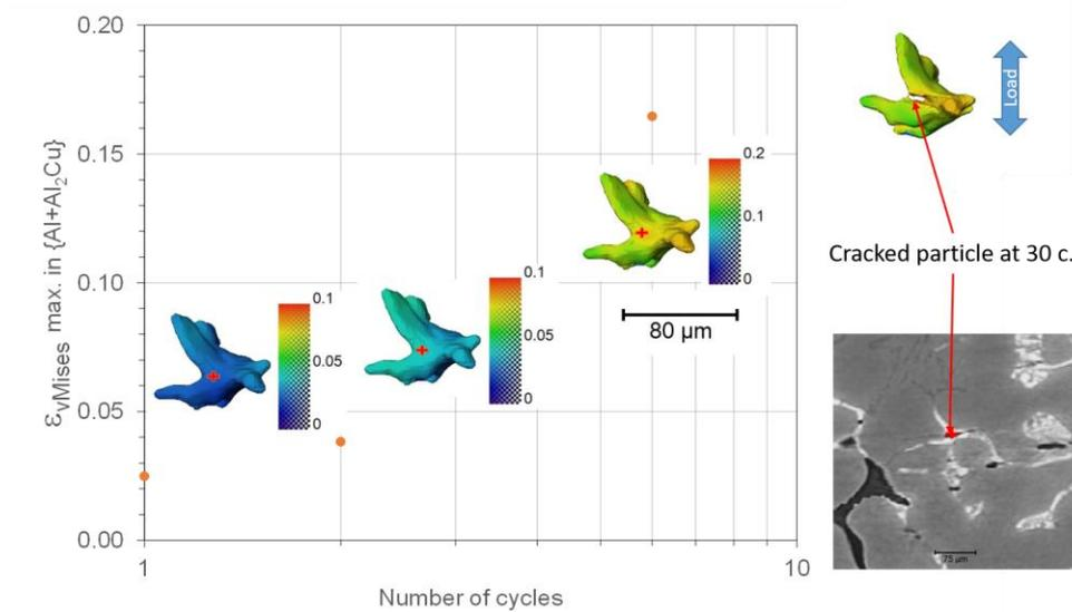
**Figure 8: Evolution of the  $\epsilon_{vMises}$  strain within one particle with the number of cycles up to the last cycle where the particle is intact. A red cross on the 3D particle, which is coloured by the strain field at the corresponding cycle, indicates the measurement location. On the right-hand side, the broken particle after 30 cycles (sample A4) is shown in 3D and within a 2D reconstructed slice.**
