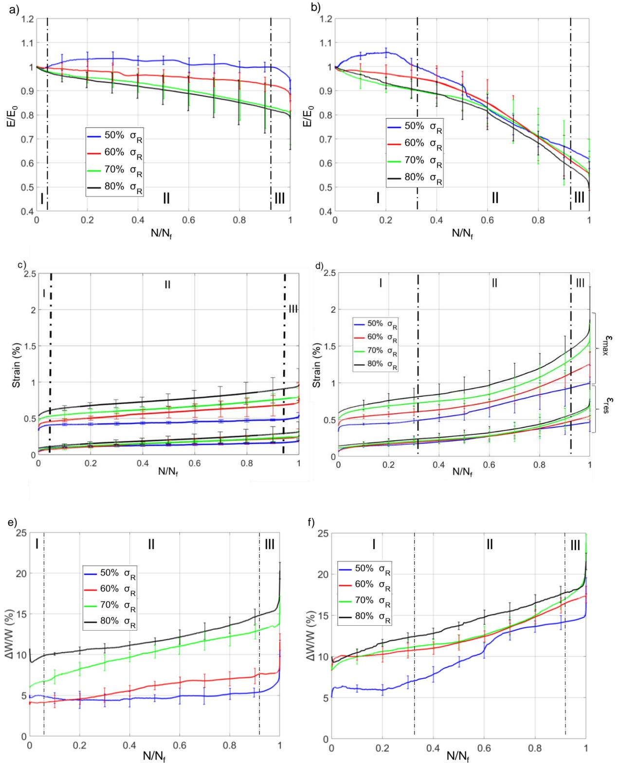
**Fig. 5.** Evolution of the mechanical parameters versus the normalized number of fatigue cycles: normalized secant modulus (a) JP\_0 (b) JP\_45, maximum and residual strains (c) JP\_0 (d) JP\_45, internal friction (e) JP\_0 (f) JP\_45.
