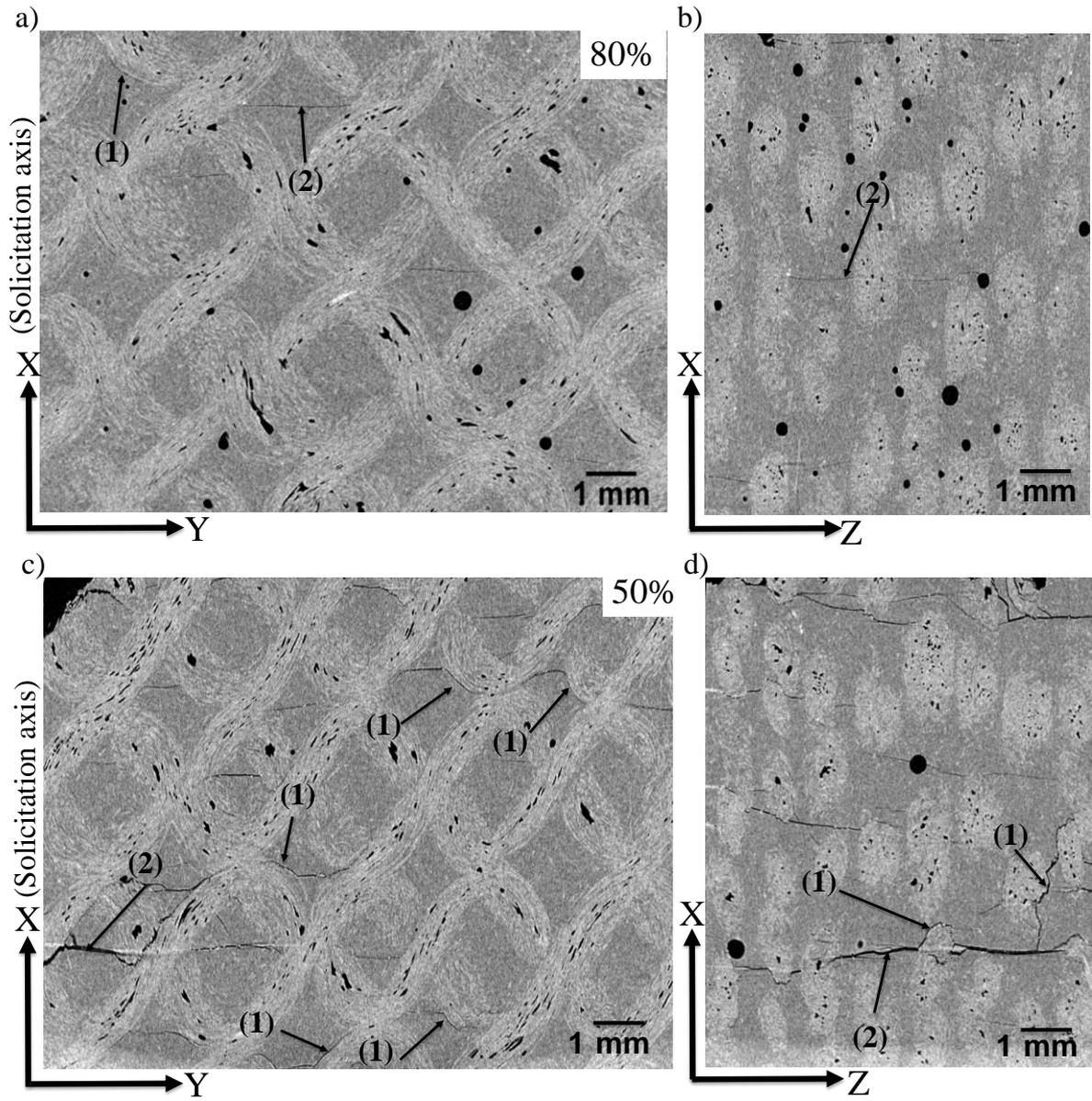
**Fig. 8.** X-ray tomography images after fatigue fracture for the JP\_45 specimens: 80%  $\sigma_R$  (a and b), 50%  $\sigma_R$  (c and d). (1) yarn/matrix debonding and (2) matrix crack, dark points are voids due to residual air bubbles in the resin.
