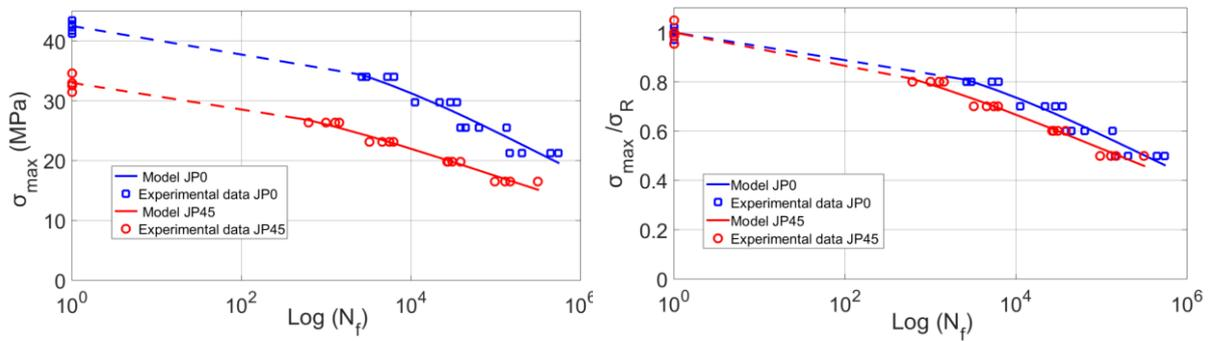
**Fig. 3.** Fatigue lifetimes diagrams (S-N curves): experimental data and D'Amore modeling for the two lay-ups: a)  $\sigma_{\max}$  as a function of  $\log(N_f)$ , b) normalized stress as a function of  $\log(N_f)$  (the coefficient of correlation  $R^2 = 0.945$  and  $0.982$  for JP\_0 and JP\_45 composites respectively).
