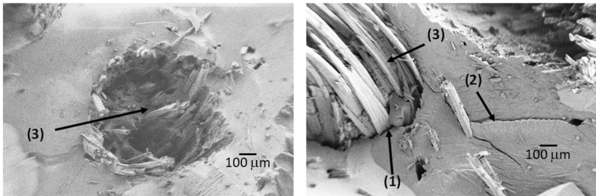
**Fig. 6.** SEM observations of the fracture surfaces for samples solicited at 80% of  $\sigma_R$ : right JP\_0, left JP\_45. (1) fiber/matrix debonding, (2) matrix cracking, (3) fiber breakage and pull-out.
