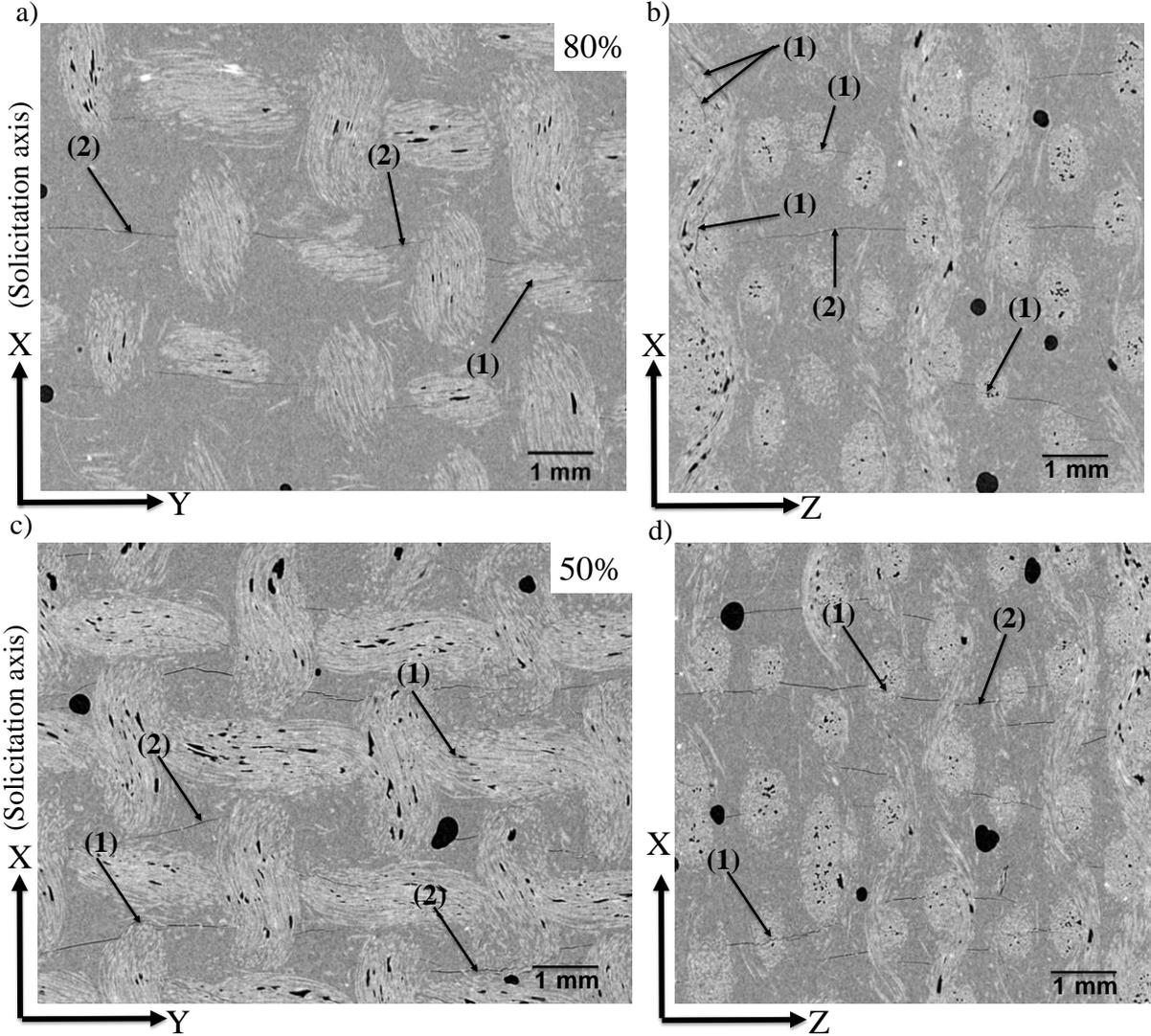
**Fig. 7.** X-ray tomography images after fatigue fracture for JP\_0 specimens: 80%  $\sigma_R$  (a and b), 50%  $\sigma_R$  (c and d), (1) yarn/matrix debonding, and (2) matrix crack, dark points are voids due to residual air bubbles in the resin.
