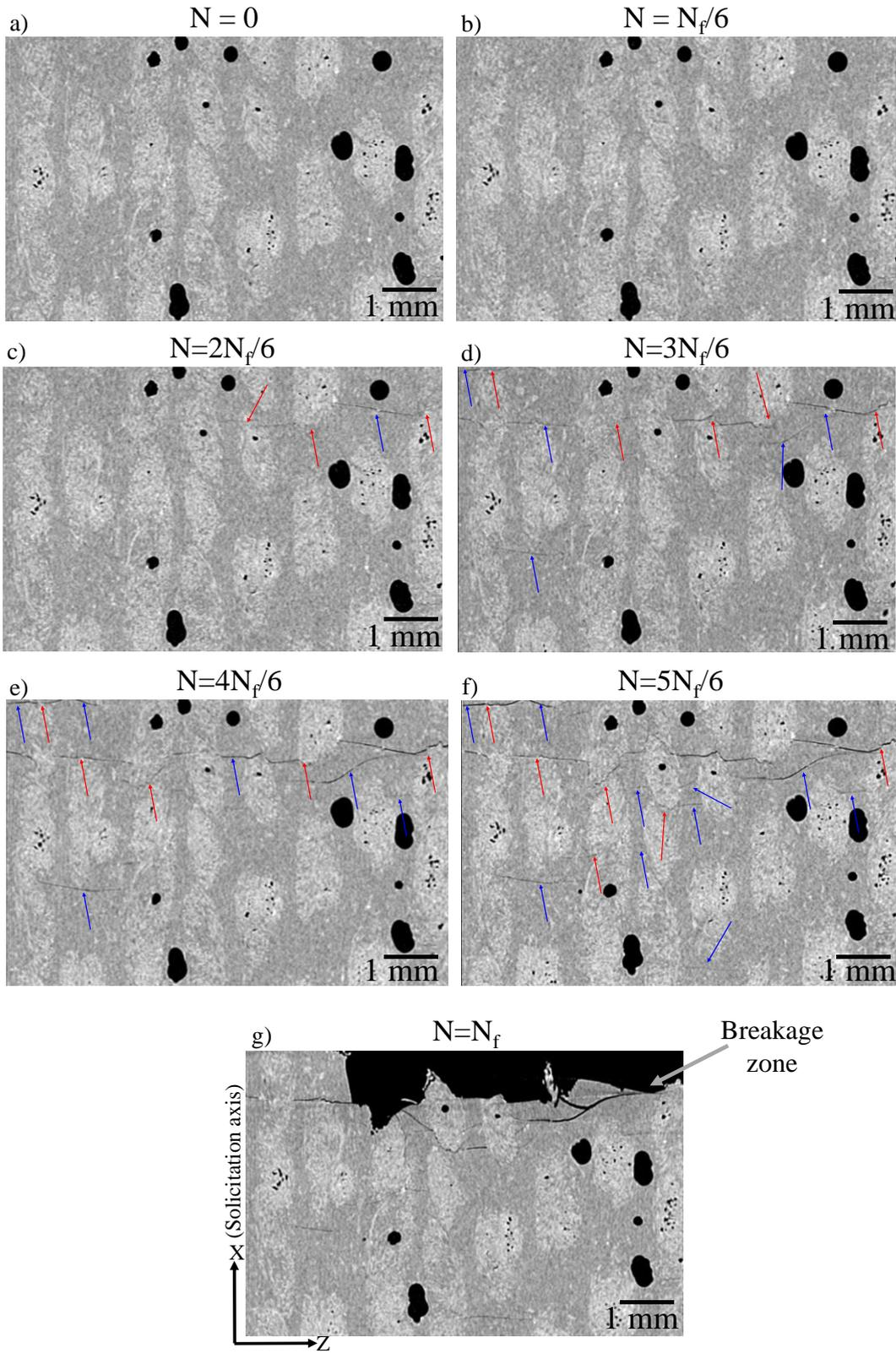
**Fig. 11.** X-ray tomography micrographs obtained for different numbers of cycles for a JP\_45 composite sample tested at 60% of  $\sigma_R$ . Red arrows indicate fiber/matrix debonding and blue ones indicate matrix cracks.
