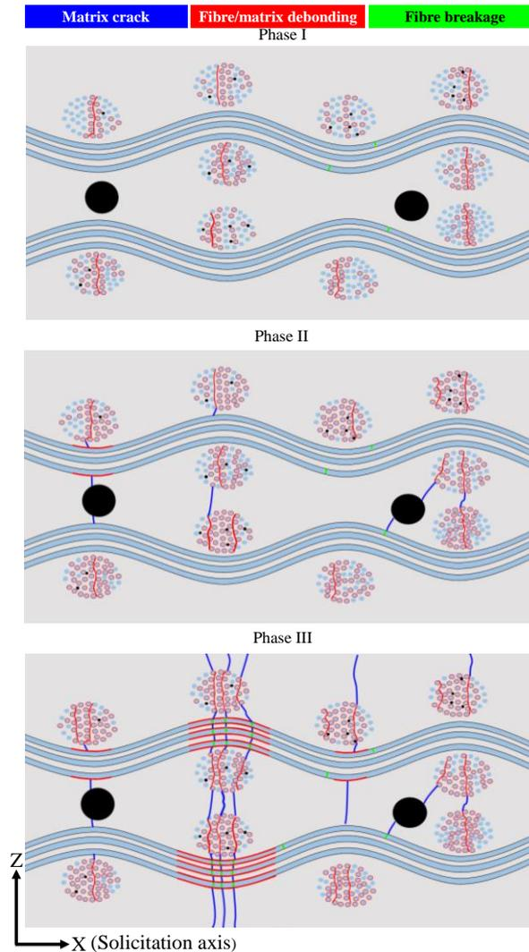
49 **Fig. 15.** Fatigue damage scenario of JP\_0 composite for low stress levels.
