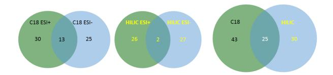
**Fig. 3.** Venn diagram analysis (Bardou et al., 2014). Comparison of number of metabolites detected by LC-MS in perilymph fluid with a C18 or a HILIC column, in positive and negative ionization mode (HESI)
