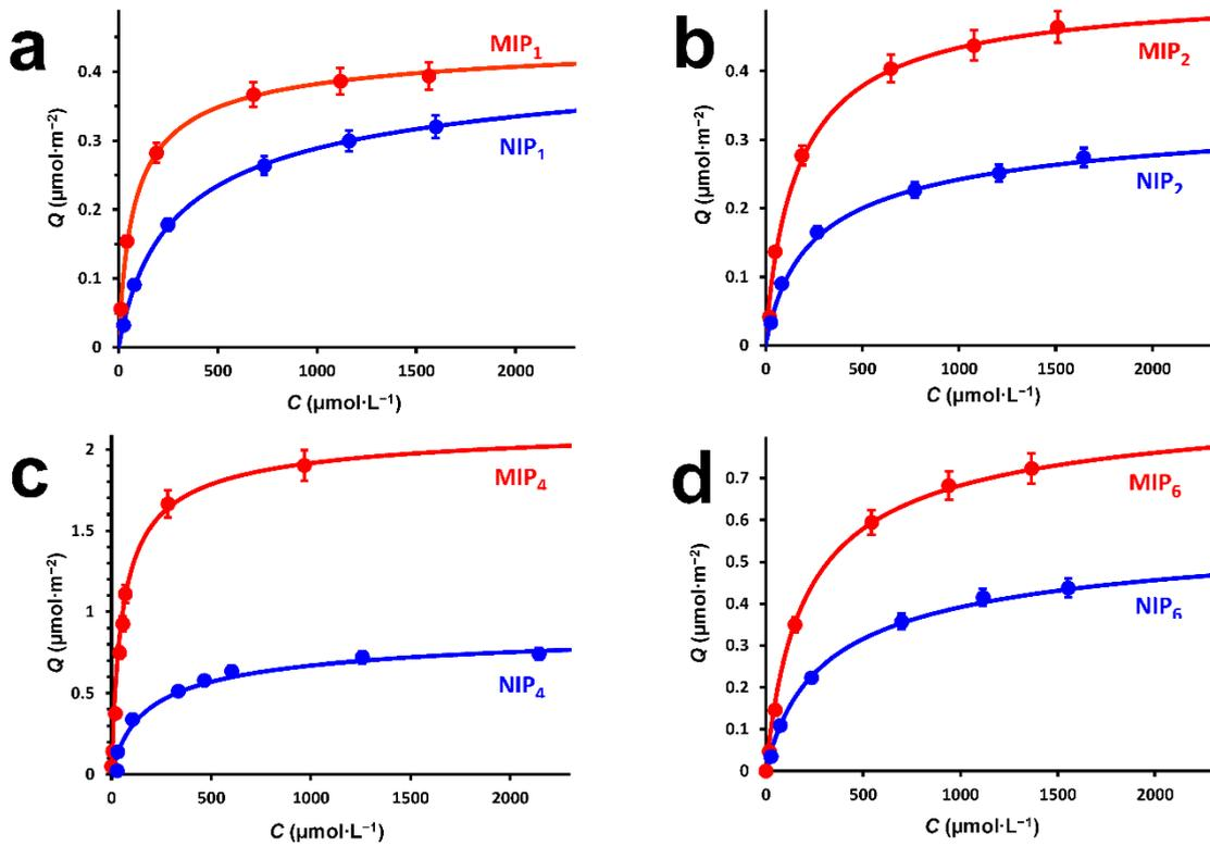
**Figure 7.** Adsorption isotherms and best fits of the adsorption models to experimental adsorption of HA onto MIP<sub>1</sub> and NIP<sub>1</sub> (a), MIP<sub>2</sub> and NIP<sub>2</sub> (b), MIP<sub>4</sub> and NIP<sub>4</sub> (c), and MIP<sub>6</sub> and NIP<sub>6</sub> (d) at 298 K and pH 5.5.
