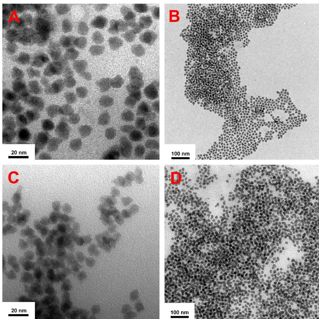
**Figure 5.** TEM images of MIP (A, B) and NIP (C, D) at two magnifications (scale bars are 20 nm and 100 nm).
