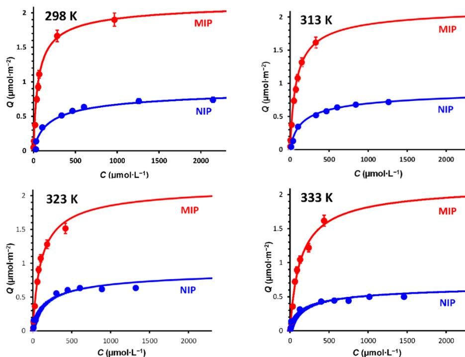
Figure S7. Adsorption isotherms of HA to MIP<sub>4</sub> and NIP<sub>4</sub> at different temperatures.
