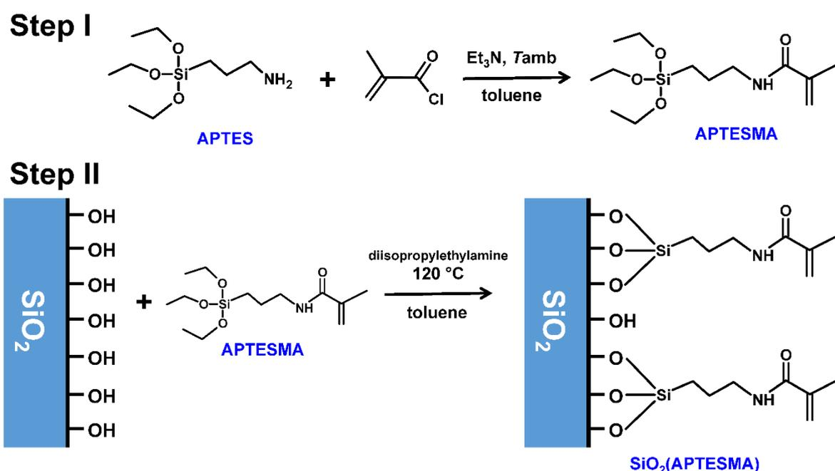
**Figure 1.** Reaction schemes for the preparation of the methacryloyl-modified silica SiO<sub>2</sub>(APTE SMA). *Step I:* Synthesis of APTE SMA. *Step II:* Grafting of APTE SMA onto the silica surface.
