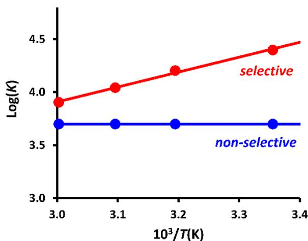
**Figure 9.** Variation of  $\text{Log}(K_a)$  as a function of  $10^3/T$  for the selective (red) and non-selective (blue) adsorption of HA on the imprinted material MIP<sub>4</sub>.
