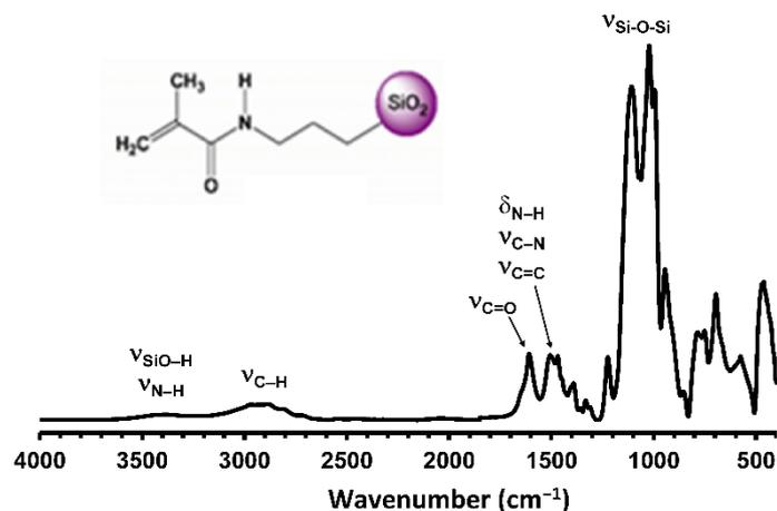
Figure S1. IR spectrum of SiO<sub>2</sub>(APTESMA).
