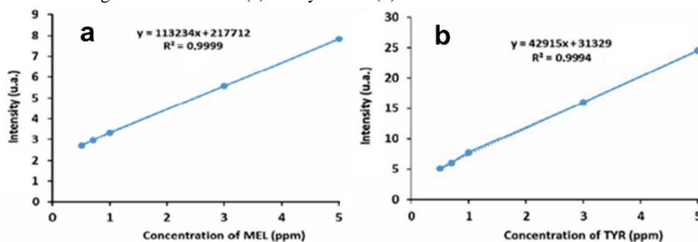
Figure S11. Calibration curve for melamine (a) and tyramine (b) from  $0.5$  to  $5 \text{ ppm}$ .
