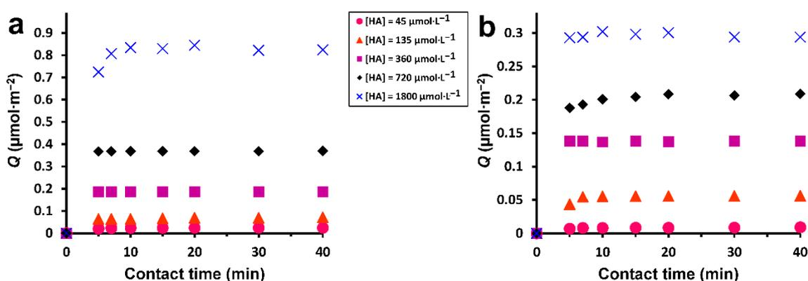
**Figure 10.** Kinetics of HA adsorption on MIP<sub>4</sub> (a) and NIP<sub>4</sub> (b) for five HA concentrations at pH 5.5.
