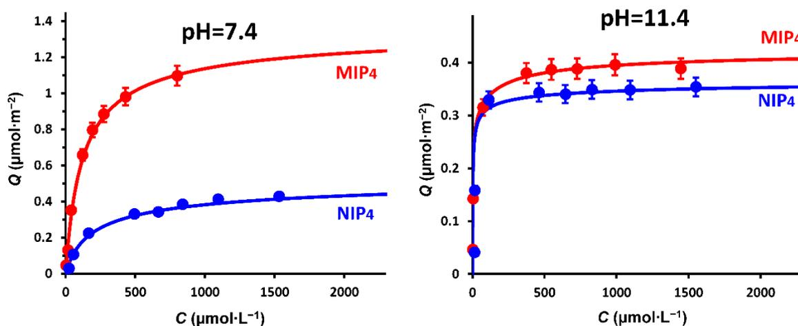
**Figure 8.** Adsorption isotherms of HA to MIP<sub>4</sub> and NIP<sub>4</sub> at 298 K and pH 7.4 and 11.4.
