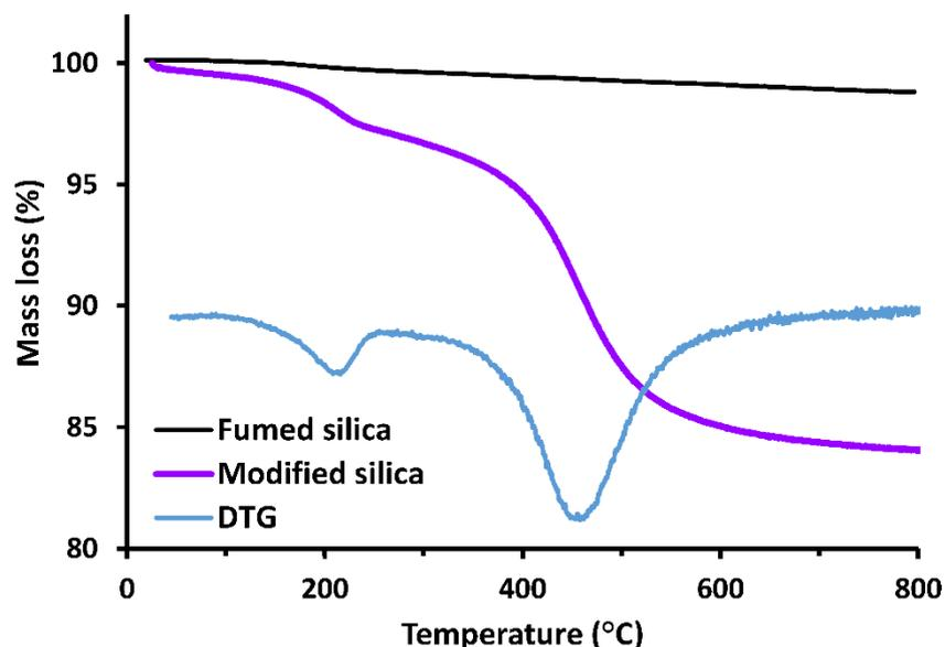
**Figure S4.** Thermogravimetric analyses of SiO<sub>2</sub>(APTESMA) and starting fumed silica. DTG is the derivative of the mass loss of modified silica with respect to temperature.
