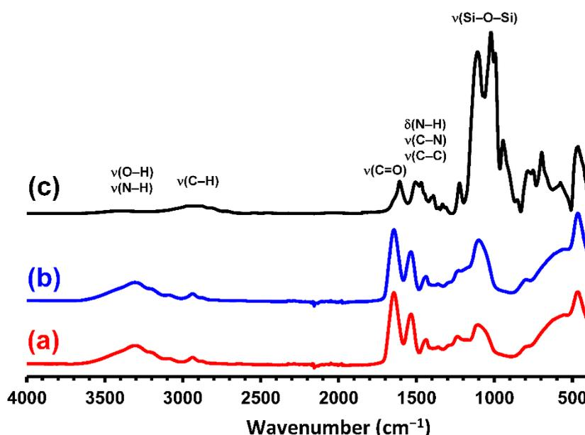
**Figure 3.** IR spectra of MIP<sub>4</sub> (a), NIP<sub>4</sub> (b), and SiO<sub>2</sub>(APTESMA) modified silica (c).
