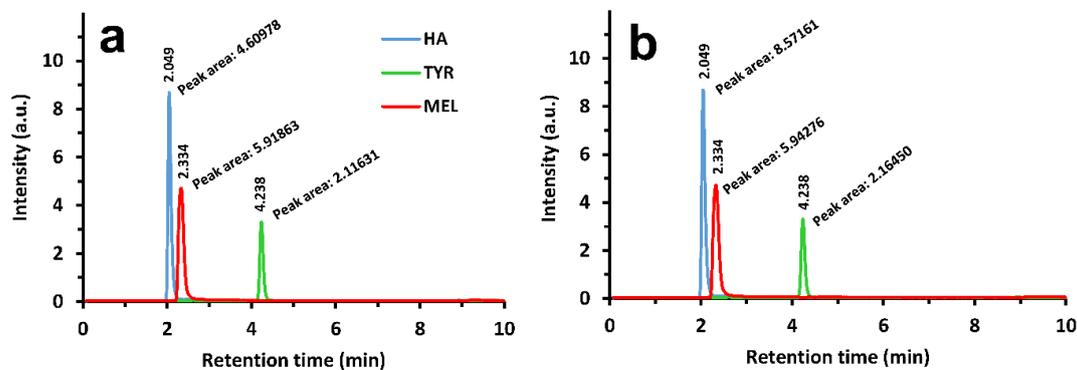
Figure S12. Chromatograms of HA (blue), MEL (red) and TYR (green) for analysis of adsorption to MIP<sub>4</sub> (a) and NIP<sub>4</sub> (b).
