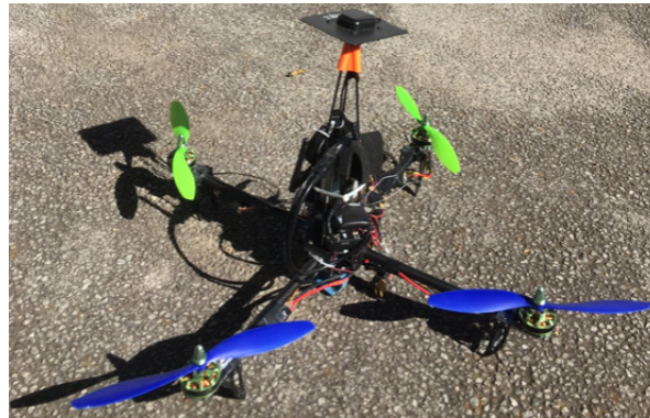
Figure 11. X4-prototype setup with the embedded control system.
