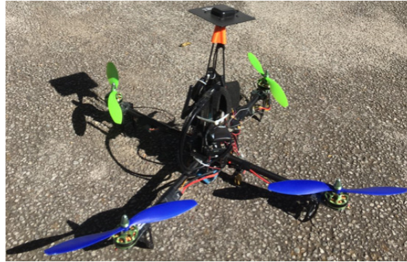
Figure 11. X4-prototype setup with the embedded control system.
