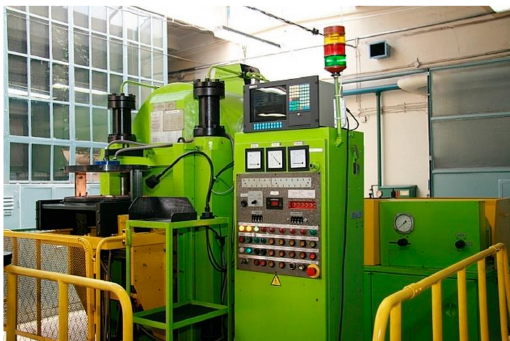
Figure 9. HP-SPS device at the Institute of Advanced Manufacturing Technology (at Krakow) in Poland (from [57]).
