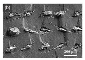
Figure 10. Scanning electron micrographs of the fracture surfaces of printed bars (1-core filaments) (a) without CIP after printing and (b) with CIP. Isostatic pressing helps to close pores trapped between the printed lines and is used for all the bars tested in this work.
