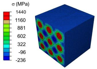
Figure 11. Finite element calculations of thermal stresses parallel to the steel fibers after cooling from  $1400\,^{\circ}\text{C}$  in a composite fabricated with a 1-core filament. A compressive stress develops in the alumina matrix.
