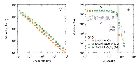
Figure 2. Rheology of the pastes used in the printing process. (a) Variation of the viscosity with shear rate. The viscosity of the pastes and their shear thinning coefficients match  $(n\sim0.1)$ . (b) The viscoelastic response of the pastes also matches.
