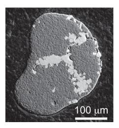
Figure 9. Cross sections of sintered filaments with 3 cores. In this system the metallic cores are highly distorted during extrusion.
