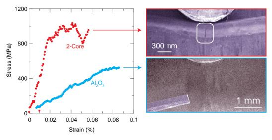
Figure 5. Bending of single filaments. Alumina filaments are brittle. The addition of the steel cores increases the bending strengths and prevent brittle filament failure.
