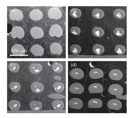
Figure 4. Polished cross sections of a sintered woodpile structure fabricated using: (a) alumina filaments; (b) 1-core, (c) 2-core and (d) 1-core with a porous interlayer (generated using a  $C-Al_2O_3$  ink, 10/90 in vol) filaments. The steel is visible as the brighter phase in the filaments.
