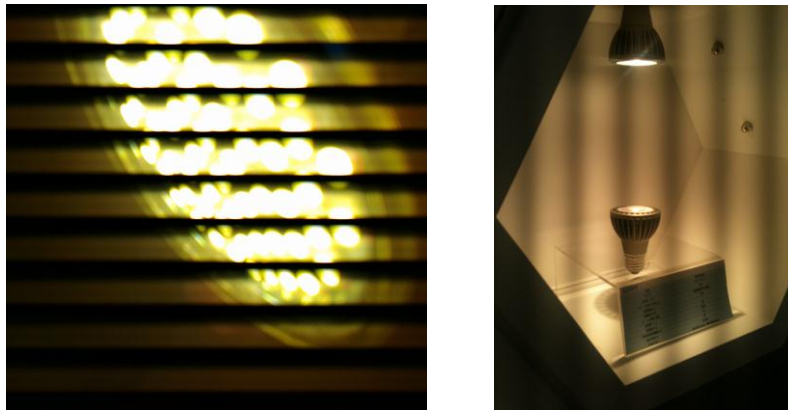
Figure 9: Flicker detection using the built-in camera of a cellular phone obtained by LAPLACE. Flicker is leading to the appearance of dark fringes in the image.
