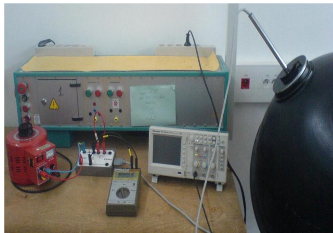
Figure 6: Diagram of the flicker measuring set up in LAPLACE
