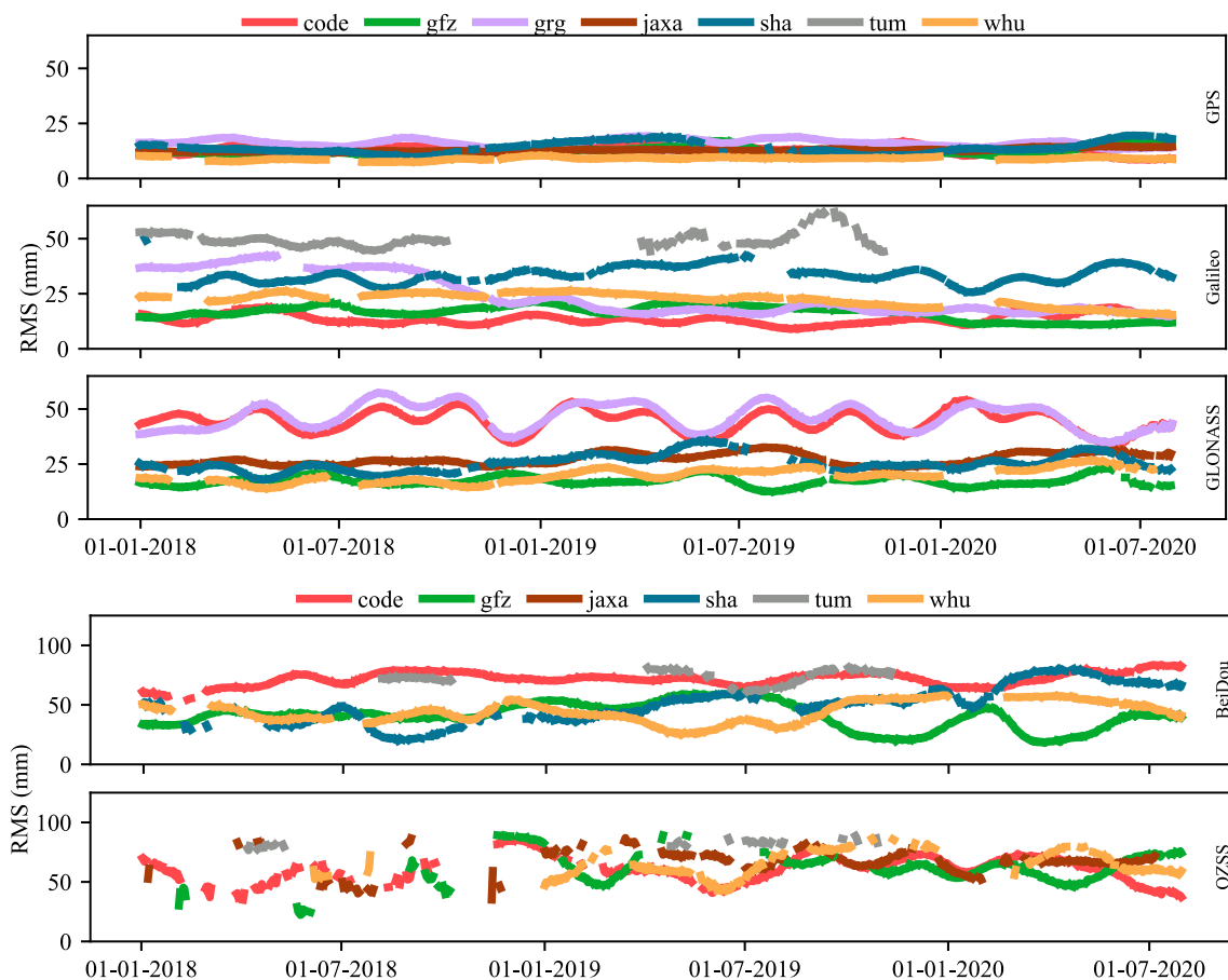
Fig. 2 Constellation-specific RMS differences between the individual AC orbits and the combined solution for AC plus constellation weighting
