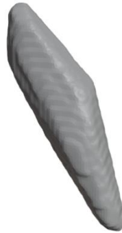
Figure 10: 3D mesh of a simulated PVD column
