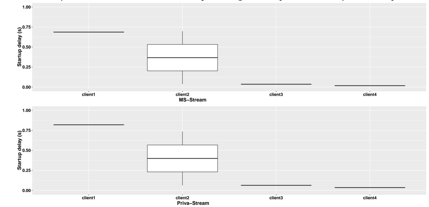
Startup delay (s) - MS-Stream (top) vs PRIVA-STREAM (bottom)
