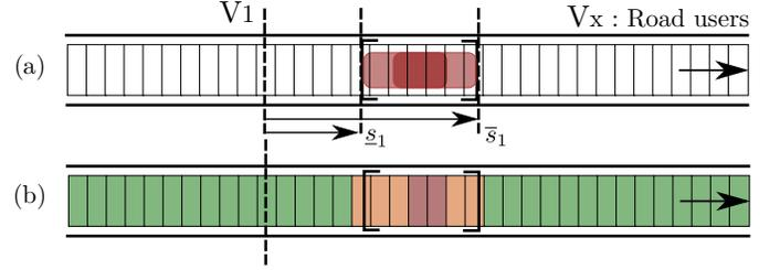
Fig. 15: Illustration of prediction stages with occupancy prediction at time horizon  $\Delta t$ . (a) Model-based object prediction with upper and lower bounds and with an overlap. The footprint of the vehicle is shown at the two ends of the reachable set. (b) Final predicted  $LGM(t_0 + \Delta t|t_0)$  with an additional occupied state in red.
