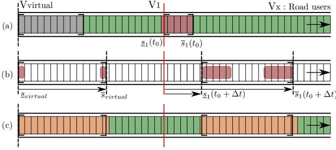
Fig. 10: Processes for building a predicted  $LGM(t_0 + \Delta t|t)$  with a virtual and a real road user. (a)  $LGM(t_0)$  with free (green), hidden (gray) and occupied (red) cells. The rear boundary of vehicle  $V_1$  is represented by a dotted line. (b) Upper and lower bounds of the predicted road users. (c) The predicted LGM is updated in orange with possibly occupied states.
