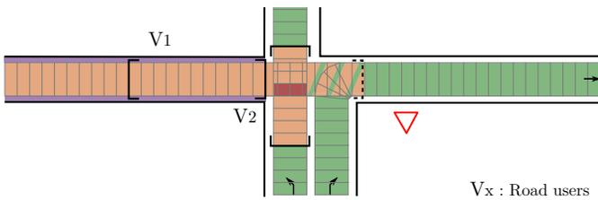
Fig. 16: Backward propagation of the neutralized constraint on a predicted LGM at time  $t_0 + \Delta t$ . The purple area remains neutralized since  $V_2$  is guaranteed to occupy at least one cell (in red) of the crossing area during the entire prediction horizon. The hatched area is therefore removed, since these cells are no longer reachable.
