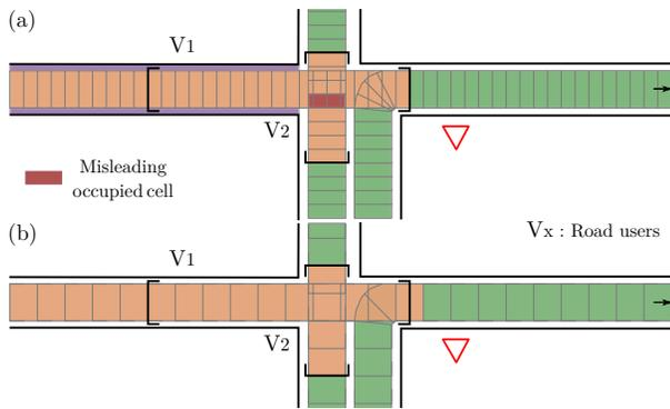
Fig. 17: Two  $LGM(t|t_0)$  computed with different sampling steps. As the sampling step increases, the misleading information due to a prediction error disappears. The situation is therefore no longer considered neutralized.
