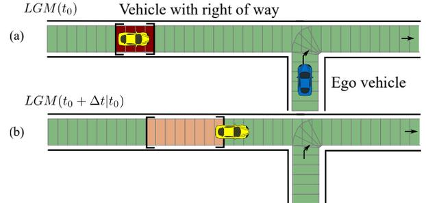
Fig. 1: At the current time  $t_0$ , the ego vehicle has a grid-based representation of the situation with free (green) and occupied (red) spaces (a). To turn right, it needs to predict the evolution of the situation at a future time  $t_0 + \Delta t$ . In situation (b), the prediction is misleading as the true position of the yellow vehicle is outside of the bounds of the reachable orange area.
