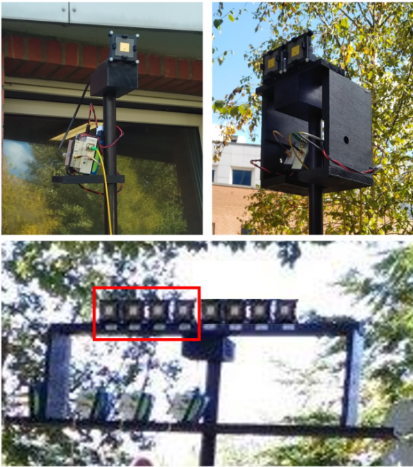
Fig. 4. Setup of the investigated linear array configurations with 1, 2, and 8 patch antennas per AP. The red box indicates a 4-antenna AP as a subset of the 8-antenna AP
