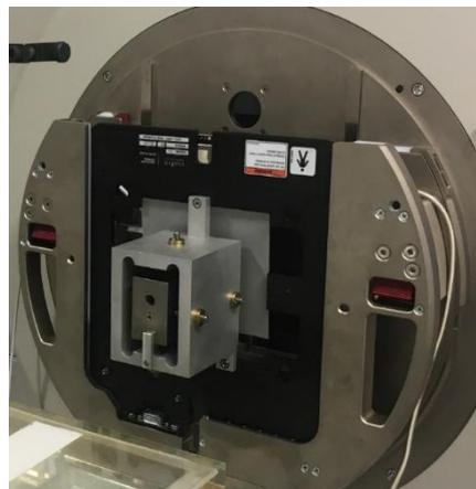
**Figure 2.** Tungsten circular collimator mounted on the exit of the treatment head.
