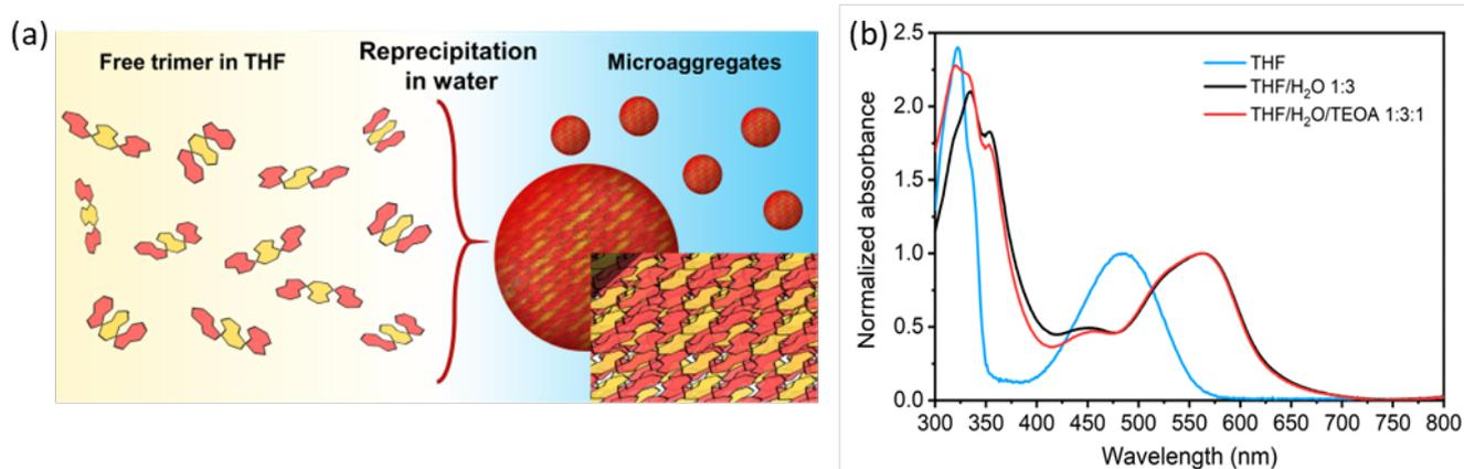
**Figure 2.** (a) The scheme of the reprecipitation method. (b) Normalized absorption spectra of EBE in THF (OD < 0.1), and of EBE in THF/H<sub>2</sub>O 1:3 (volume ratio) and THF/H<sub>2</sub>O/TEOA 1:3:1 (volume ratio), after a line subtraction treatment.
