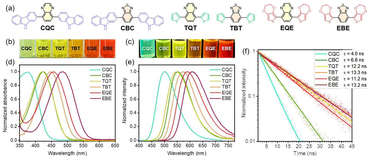
**Figure 1.** (a) Structural formulas of trimer photocatalysts. Photograph of catalysts in THF solution (b) under ambient light and (c) under UV light ( $\lambda = 365$  nm). (d) Normalized UV-Vis absorption spectra of catalysts dissolved in THF. (e) Normalized steady-state photoluminescence spectra of trimers in THF. (f) Fluorescence decays obtained by time-resolved fluorescence spectroscopy with a streak camera (in photon counting mode), fitted by a monoexponential function.
