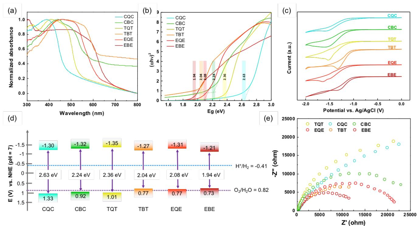
**Figure 4.** (a) DRS absorption spectra of the samples measured in the solid state (normalized intensities); (b) Calculated band gap from Tauc plots; (c) Cyclic voltammety plots (reduction scans) of trimers in acetonitrile solution and 0.1 M tetrabutylammonium perchlorate; (d) Experimentally determined HOMO and LUMO energy levels of samples; (f) Nyquist plots of EIS for trimers/FTO electrodes under UV-Vis light irradiation.
