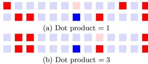
Fig. 4: Dot product of clustering labels for two traces (top and bottom). Bottom: labels for a reference trace (fixed). Top: labels of a trace to be re-aligned to the ref. trace; they are rotated to find the best candidate (*i.e.* largest dot product result). Red squares: coefficients  $-1$ , blue squares: coefficients in  $\{0, 1\}$ . More vivid colors: clustering labels 1, light tone colors: labels 0.
