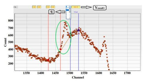
Fig. 8. Polynomial background determined for the spectrum of Fig. 7c, obtained with the proton beam aligned with the Si substrate (100) direction.
