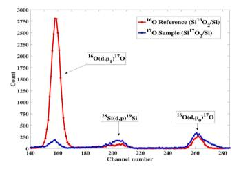
**Fig. 5.** Typical NRA spectra obtained from the <sup>17</sup>O enriched silica layer used for the cross section measurements, and a reference thin silica layer of natural isotopic composition.
