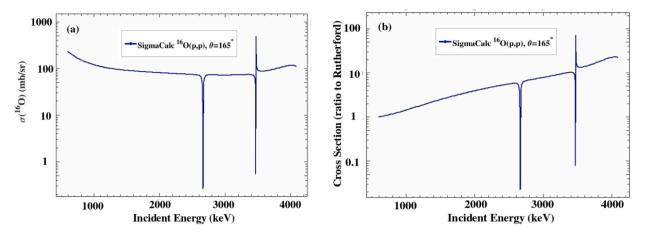
Fig. 1. a) cross section and b) the ratio to the Rutherford cross section of  ${}^{16}O(p,p){}^{16}O$  at 165 (sigmacalc) [4].
