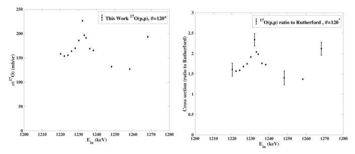
Fig. 12. a) Proton scattering cross-sections and b) the ratio to the Rutherford cross section of  ${}^{17}O(p,p){}^{17}O$  at 120° for  $E_p = 1.2-1.3$  MeV in the laboratory system.
