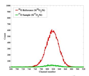
**Fig. 4.** The typical measured p-NRA spectra obtained from the <sup>17</sup>O enriched silica layer used for the cross section measurements, and a reference thin silica layer of natural isotopic composition at scattering angle  $150^{\circ}$  and Ep = 830 keV.
