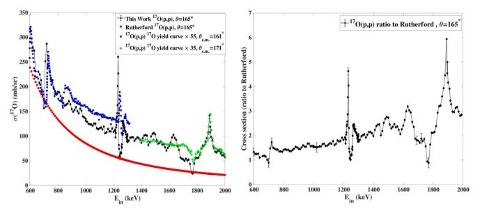
Fig. 9. a) Our measured proton elastic scattering cross-section, compared with scaled yield curves from Ref. [8,9]. b) The ratio to the Rutherford cross section of <sup>17</sup>O at 165° for  $E_p = 0.6-2$  MeV in the laboratory system. The representative uncertainty bars in b) represent the statistical uncertainty.
