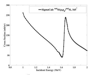
Fig. 6. <sup>nat</sup>Si(p,p) differential cross section curve.
