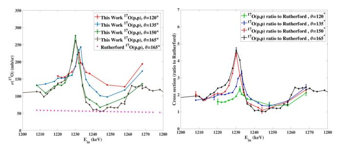
Fig. 13. Comparison of a) proton scattering cross-sections and b) the ratio to the Rutherford cross section of  ${}^{17}O(p,p){}^{17}O$  at different angles for  $E_p = 1.2-1.3$  MeV in the laboratory system.
