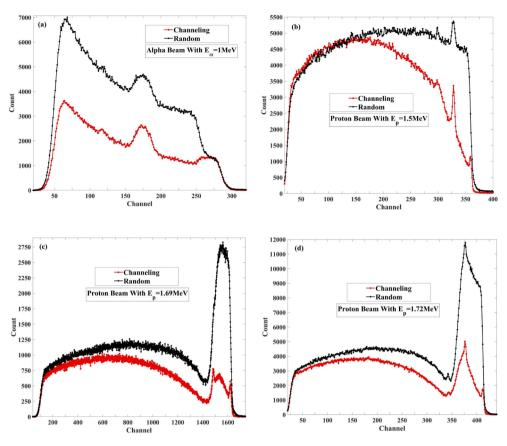
Fig. 7. The comparison between channelling and random peak at different with a) alpha beam with  $E_{\alpha} = 1$  MeV, and proton beam with b)  $E_p = 1.5$  MeV, c)  $E_p = 1.69$  MeV and d)  $E_p = 1.72$  MeV.
