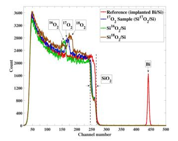
Fig. 3. The typical measured RBS spectra of the three isotopically enriched oxide targets and the Bi reference at scattering angle  $165^\circ$  and  $E_\alpha=1.8$  MeV.
