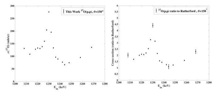
Fig. 10. a) Proton scattering cross-sections and b) the ratio to the Rutherford cross section of  ${}^{17}O(p,p){}^{17}O$  at 150° for  $E_p = 1.2-1.3$  MeV in the laboratory system.
