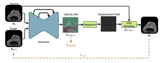
Figure 2: Unsupervised 2D intensity-based registration model between two successive slices  $\mathbf{x}_k$  and  $\mathbf{x}_{k+1}$ . Please refer to the text for complete description of notations.
