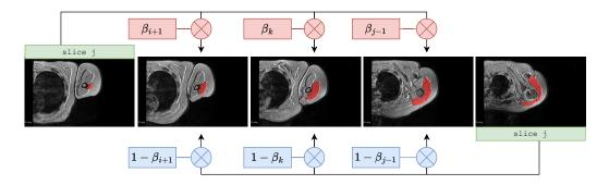
Figure 3: Label propagation framework scheme. Labels are propagated in both direction, resulting in two prediction for intermediate slices, that are fused using a weighting function  $\beta$ . Please refer to the text for complete description of notations.
