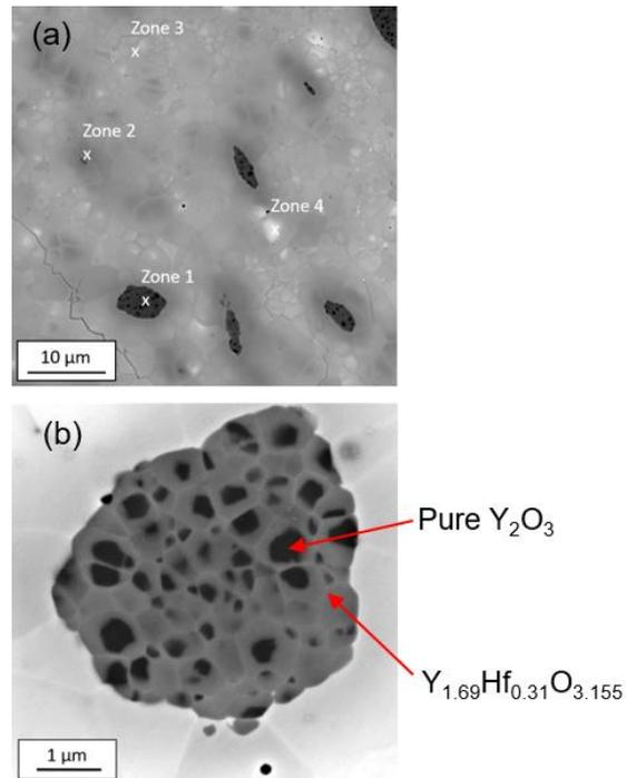
Figure 8: SEM-BSE observations of the 33YSHf sample sintered using SPS at 1750 °C: (a) observation of four contrasted zones, corresponding to different chemical compositions and (b) zoom on the zone 1: black spots inside the dark nuance corresponding to pure Y<sub>2</sub>O<sub>3</sub>.
