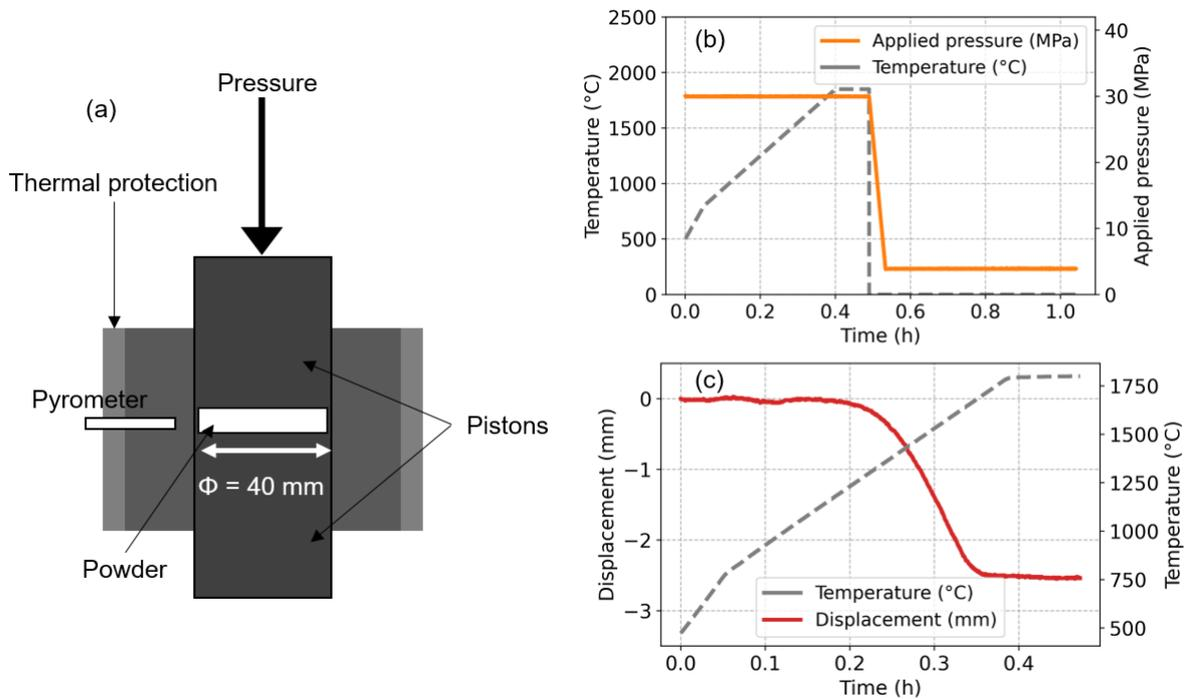
Figure 2: (a) Schematic view of the graphite die, (b) a typical sintering cycle and (c) a representative displacement curve of the sample 50YSHf - 1800  $^{\circ}$ C, versus time as a function of the temperature (measured by a pyrometer).
