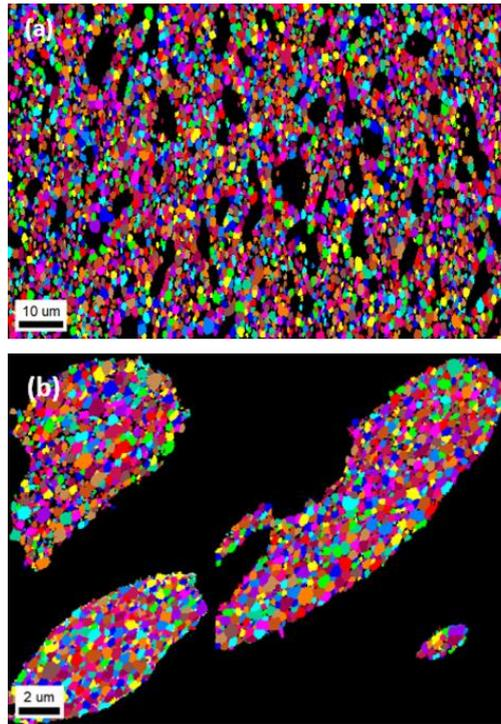
Figure 9: Representative EBSD analysis (grain maps) of a sintered sample (40YSHf, 1650 °C) at two different scales (a) HfO<sub>2</sub>-rich zones and (b) zoom on dark areas of an Y<sub>2</sub>O<sub>3</sub>-rich zone.
