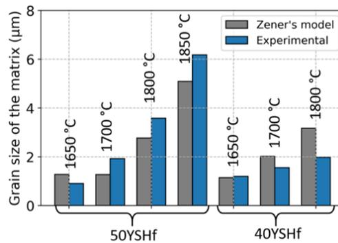
Figure 13: Comparison between the grain size of the matrix for 40YSHf and 50YSHf samples using the Zener's model (based on the experimental size of the secondary phase obtained by EBSD analysis and the experimental volume fraction of the phases determined from XRD analysis) and the experimental size of the matrix (obtained by EBSD analysis).
