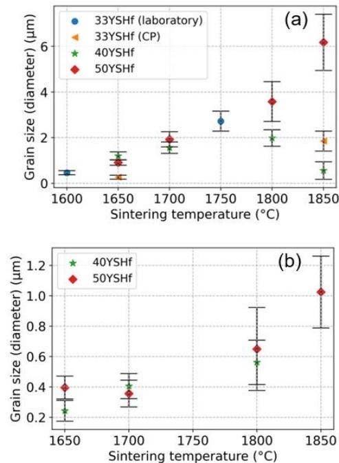
Figure 10: Grain size evolution with sintering temperature, from the EBSD analysis for (a) the population of the coarsest grain size ( $Y_2Hf_2O_7$  phase) and (b) the population of the smallest grain size ( $Y_2O_3$ -rich phases).
