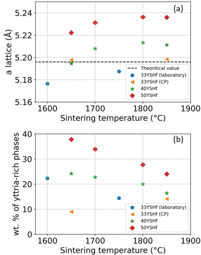
Figure 6: (a) Evolution of the lattice parameter of the cubic  $Y_2Hf_2O_7$  phase with the sintering temperature for yttria containing compositions (CP indicates the commercial powder) and (b) evolution of the proportion of the yttria rich phases ( $Y_{1.69}Hf_{0.31}O_{3.155}$  and  $Y_2O_3$ ) with the increase in sintering temperature for different amounts of  $Y_2O_3$  in  $HfO_2$ .
