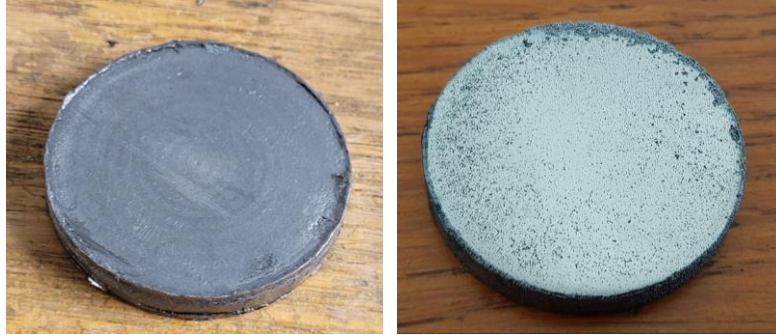
Figure 4: Sample before (left) and after (right) first coarse polishing
