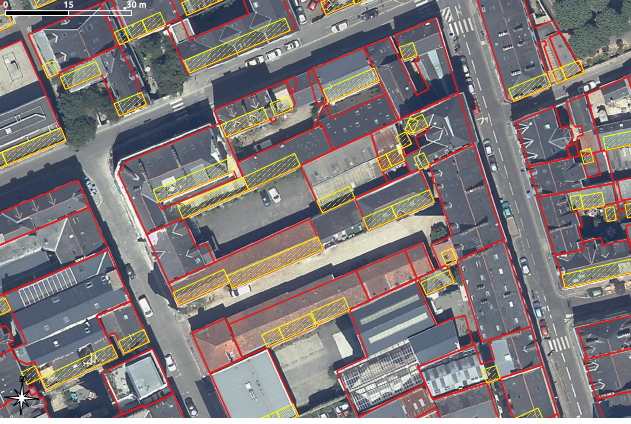
Figure 5: Above the well-aligned facade is a 3.2 m deep roof ribbon (yellow shaded polygon) on which a GENESIS green node may be potentially installed. To avoid the sun shading effect, we removed any part of the roof ribbon that protruded beyond the party wall. Red polygons correspond to building footprints in the terrain data (BD Topo®).
