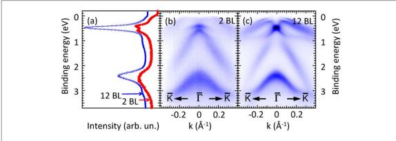
**Figure 5.** (a) Valence band PES spectra at normal emission of InAs(1 1 1)A covered by 2 and 12 BL Bi. (b) and (c) corresponding ARPES spectra along the  $\overline{\Gamma}$ - $\overline{K}$  direction. Spectra were recorded at  $h\nu=20$  eV.
