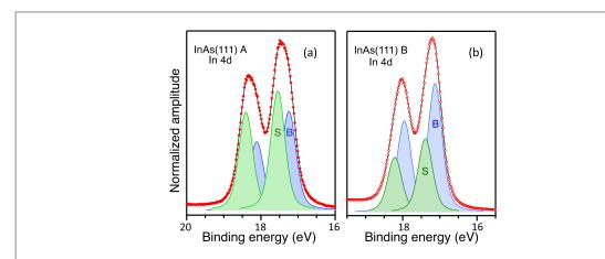
**Figure 2.** In 4d PES spectra of clean InAs(1 1 1): (a) A side; (b) B side. Raw data are shown as dots; the lines are the fit to the data and the components (denoted by B for the bulk and by S for the surface) involved in the fit.
