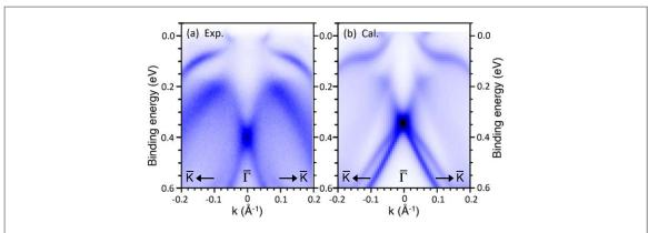
**Figure 6.** Bi(1 1 1) ARPES spectrum along the  $\overline{\Gamma}$ – $\overline{K}$  direction. (a) Experimental data, taken at  $h\nu=20$  eV, for 12 BL Bi(1 1 1) grown on InAs(1 1 1)A. (b) Calculation for  $h\nu=22$  eV.
