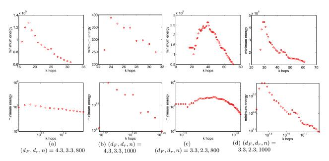
Figure 7: Minimum accumulated end-to-end energy versus hops, averaging over 100 transmitter-receiver pairs,  $\delta = 2$ , linear scale left side of sub-figures, logarithmic scale right side of sub-figures
