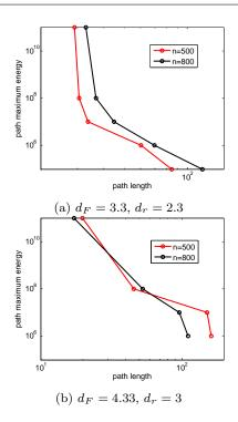
Figure 9: Path Maximum Energy trade-off with delay (i.e. path length)
