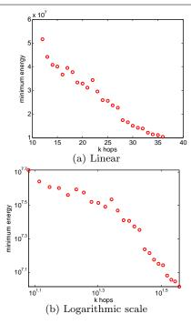
Figure 8: Minimum accumulated end-to-end energy versus hops, averaging over 100 transmitter-receiver pairs,  $\delta = 3$
