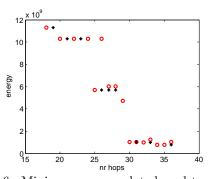
Figure 6: Minimum accumulated end-to-end energy versus hops for a transmitter-receiver pair (fixed and allowed number of hops in red circles, and maximum number of hops in black stars).
