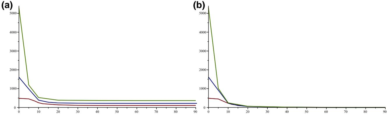
**FIGURE 15** Size of the garage set as function of coverage radius, in brown  $\theta = d_r/4$ , in blue  $\theta = 1.2d_r/4$ , and in green  $\theta = 1.4d_r/4$ . (a) Garage number in a map with border. (b) In a torus map with no border
