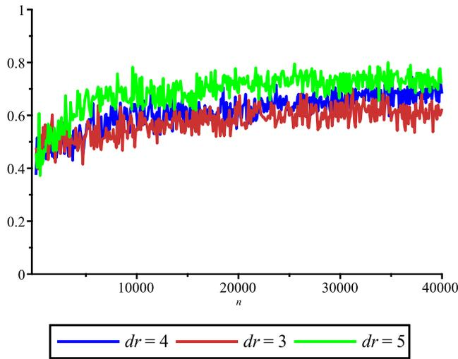
FIGURE 10 Proportion of isolated nodes for  $\theta < d_r/4$
