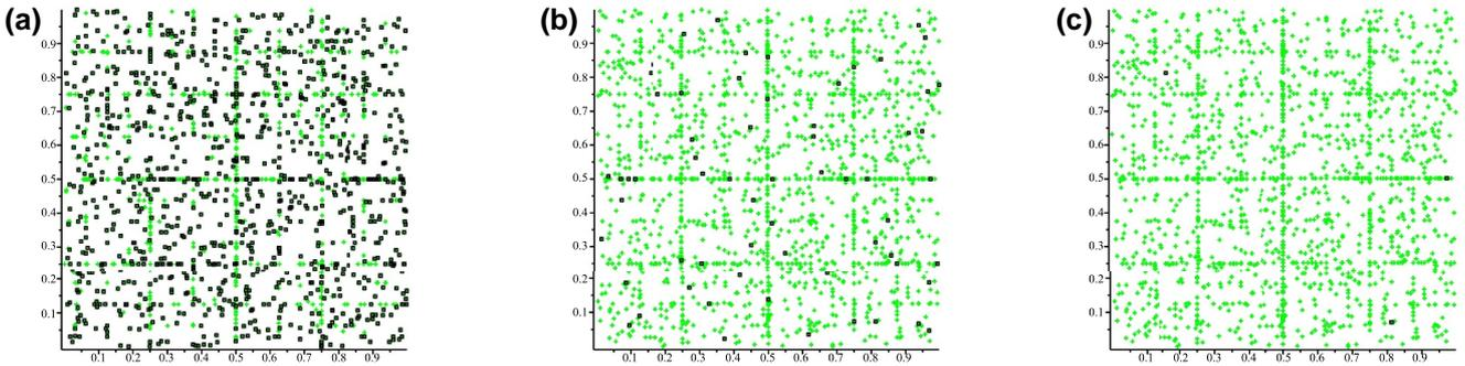
**FIGURE 16** Map of drone garages (black circles), among the base stations (green crosses), for different coverage distances in a torus map; (a) coverage distance  $5R_n$ , (b) coverage distance  $20R_n$  and (c) coverage distance  $80R_n$
