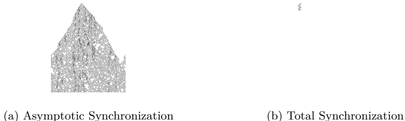
Fig. 2: Evolution of the synchronization error for elementary rule 18 with 500 cells from a single cell error ( e = 0.2\% ). The time is represented on the vertical axis. A black pixel is an erroneous cell in the synchronized CA.
