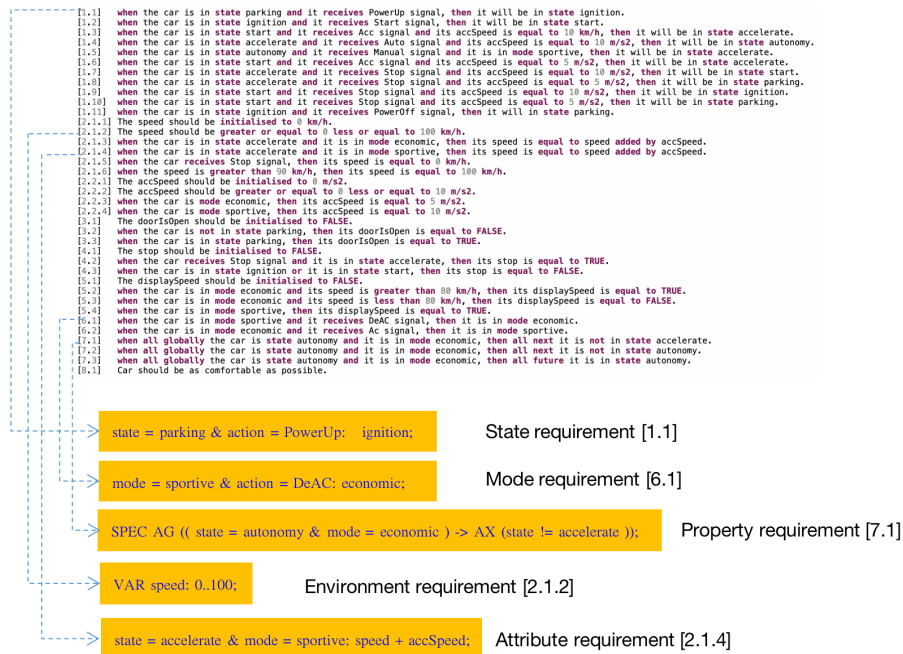
FIGURE 6: An Example of the Model Transformation
