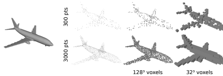
Fig. 2: Visualization of voxelizations at resolutions 32^3 and 128^3 of input point clouds with 300 and 3000 points.
