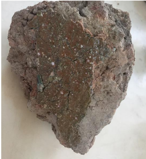
Fig. S1: View from the material which was formed on the walls inside of the kiln (left) and view from the analysis spot recorded with pXRF instrument.
