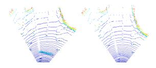
Fig. 10. The ghosting effect of a moving car is greatly reduced due to the semantic-guided moving objects segmentation and removal
