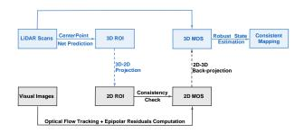
Fig. 1. Overview of the proposed LiDAR-Vision fusion approach for moving objects segmentation and state estimation
