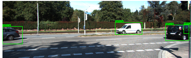
Fig. 3. The LiDAR-based 3D object detection results mapped on the image plane through the perspective projection
