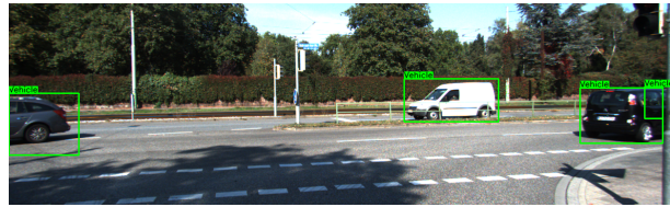
Fig. 3. The LiDAR-based 3D object detection results mapped on the image plane through the perspective projection
