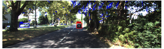
Fig. 8. The tiny moving object with degenerate motions (move along the epipolar plane) is successfully segmented with the FVB constraint
