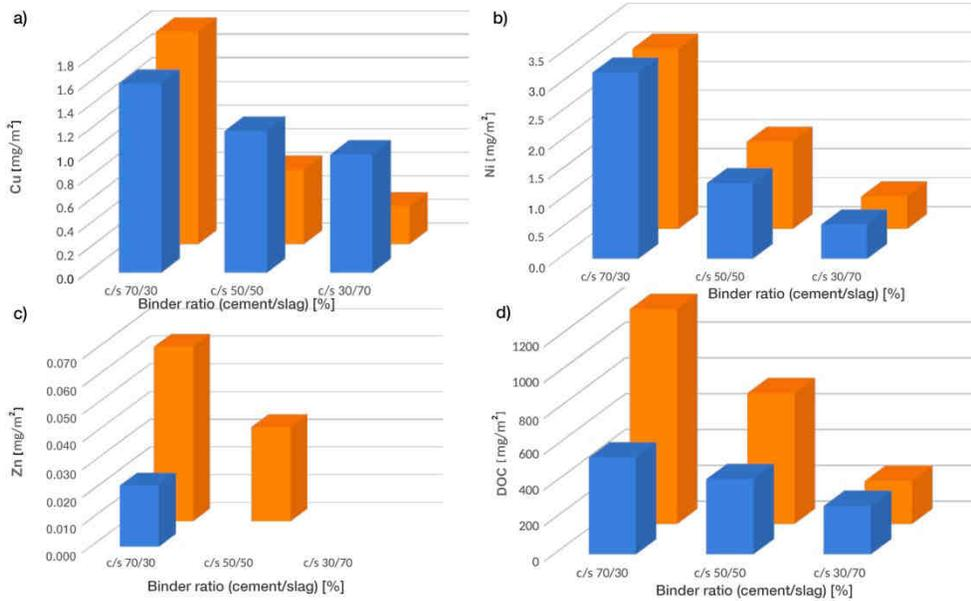
Fig. 4. Summary of the leached amount per unit area for: a) Cu, b) Ni, c) Zn and d) DOC on the day 36<sup>th</sup> for the best and worst cases. Orange colour - best case *HBLW* (High binder-Low water ratio in a stabilising mixture). Blue colour - worst case *HWLB* (High water-Low binder ratio in a stabilising mixture). Substances show a systematically decreasing trend with the increased slag content. Variations in 3 cases of bars show ratio cement/slag as 70/30 %, 50/50 % and 30/70 %
