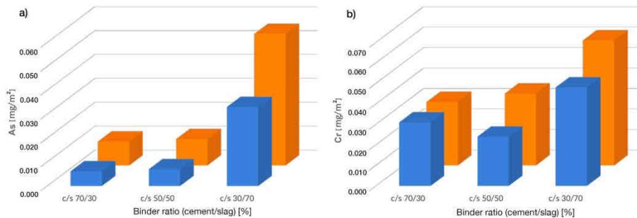
Fig. 5. Summary of leached amount for: a) As and b) Cr on day 36<sup>th</sup> for the best and worst cases. Orange colour - best case *HBLW* (High binder-Low water ratio in a stabilising mixture). Blue colour - worst case *HWLB* (High water-Low binder ratio in a stabilising mixture). Substances show a non-existent or increasing trend with increased slag content. Variations in the 3 cases of bars show proportions of cement/slag in binder ratio as 70/30 %, 50/50 % and 30/70 %
