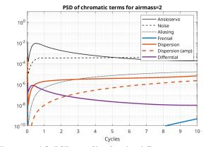
Figure 7. AO PSDs profiles for the different term in the AO error budget for a 50x50, 4kHz system under good seeing and airmass=2. We consider the worst case with  $\lambda_{SCI}$ =620nm and  $\lambda_{WFS}$ =1400nm.
