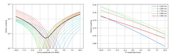
Figure 5. Sensitivity to come aberration for a spider-free VLT aperture. Coloring on the left plot follows the logic of the right plot, with finer wavelength sampling. Black curve on the left is the average over the band.
