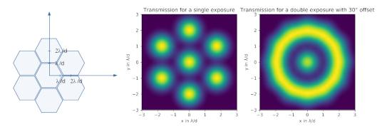
Figure 1. Left: schematic view of the RISTRETTO IFU. Midlle: transmission map due to single mode fiber coupling. Right: transmission map after  $30^{\circ}$  rotation of the IFU.
