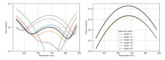
Figure 3. Stellar and planet coupling as a function of wavelength for a CaF2 PIAA. We show the case of VLT pupil (16.2% obstruction) without and with spiders, under different orientations with respect to the lenslet.
