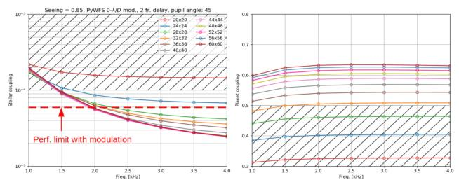
Figure 8. End-to-end RISTRETTO performance on Prox Cen as a function of loop speed. We consider a VLT pupil with spiders oriented to show an average behavior. On the left, the red dotted line shows the performance limit with modulation of  $3\lambda/D$ .
