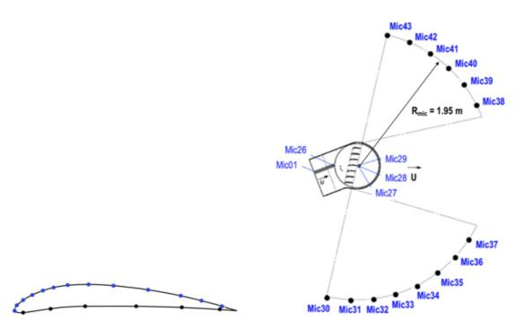
Figure 4 – Static pressure probes around the airfoil. Figure 5 – Induct mics. and farfield antenna.
