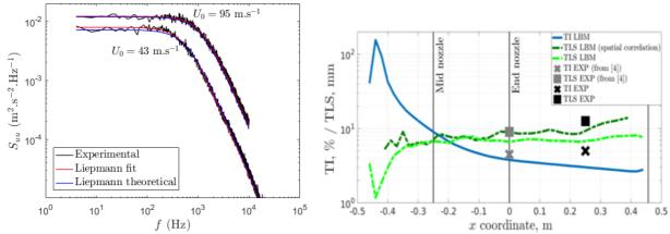
Figure 10 – Axial velocity spectra (Log scales) measured by HW and from Liepmann model.
