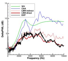
Figure 17 — DeltaPWL achieved by all methods for ON1 design and compared to experiment (Mach 0.34).
