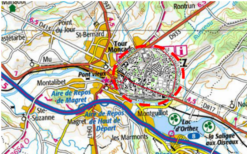
Figure 13: Example of a focus+context interface in a multi-scale map with the 1:25k map displayed inside the lens, and the 1:100k map displayed outside the moving lens.
