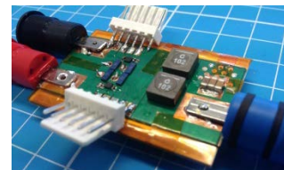
Fig. 11. Experimental converter with screen printed capacitors
